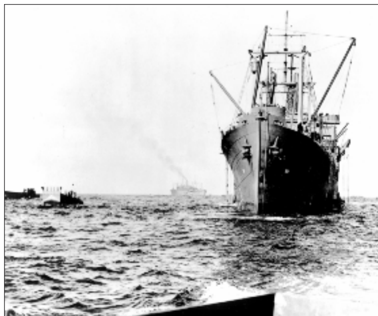
Rare photograph of the USS Hunter Liggett debarking troops for the Guadalcanal landings. Notice the use of cargo derricks to lower landing craft into the water. (Courtesy of the U.S. Navy)
