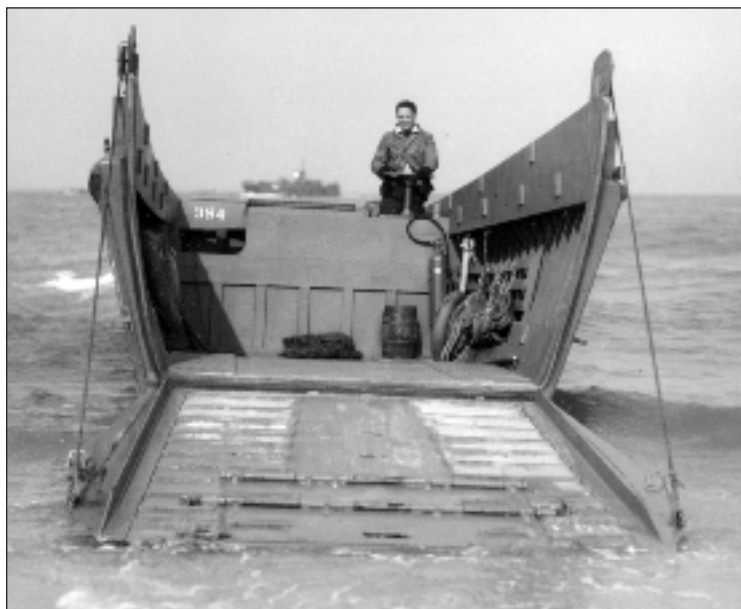
Photo showing an LCVP, which had lines similar to an LCP, or Higgins Boat, but boasted easier access between the cargo bay and the beach. (Courtesy of the U.S. Navy)
