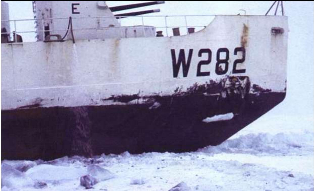
*The bow of wind class icebreaker is designed to ride up on the ice and crash down to break through the ice. This action, combined with rolling the ship by pumping water from side-to-side, allows the ship to move forward through the ice field.*
