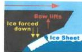
But icebreakers don't try to plow through the pack ice - they use their power and momentum to push the sloping bow up onto the ice. The great weight of the ship then pushes down on the ice, letting gravity do the heavy work.
