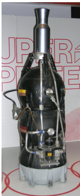
The photo at left is from the Smithsonian exhibit, donated by Aerojet, of an engine that proved the concept. A beautifully fashioned machine showing the three spheres, firing chamber and nozzle, simple, effective, setting the standard for what became extra-terrestrial flights
