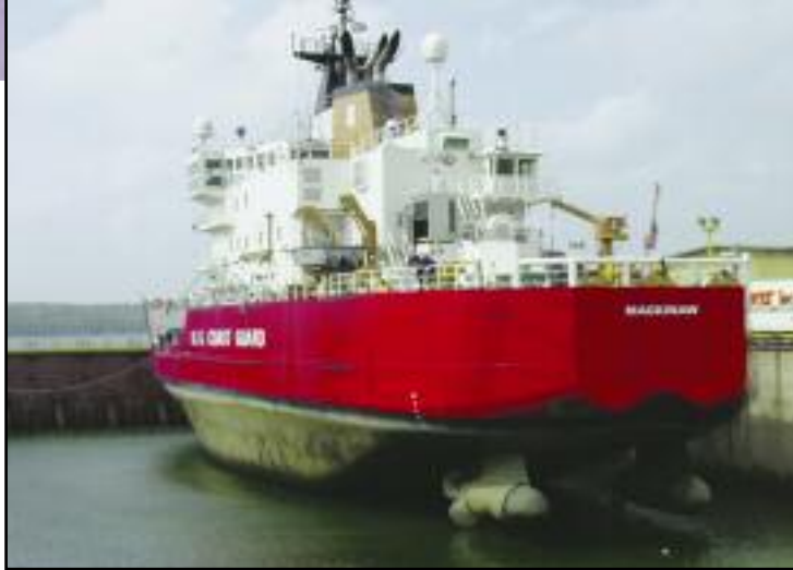
Figure 2: The USCG icebreaker Mackinaw , the first icebreaker in North America to be fitted with azimuthing podded propellers, features two Azipods® at the stern. The Mackinaw 's stern is an example of the "sledge" shape. USCG Photo.
