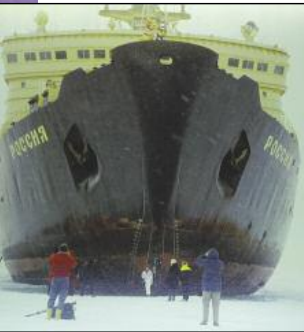
Figure 1: The Russian nuclear-powered icebreaker Rossia , shown here at the North Pole in 1990, features the classic wedge-shaped bow. Photo by A. Tunik.
