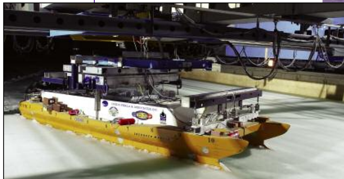
Figure 3: An ice test of a small waterplane area twin hull ferry model. Photo courtesy U.S. Navy.
