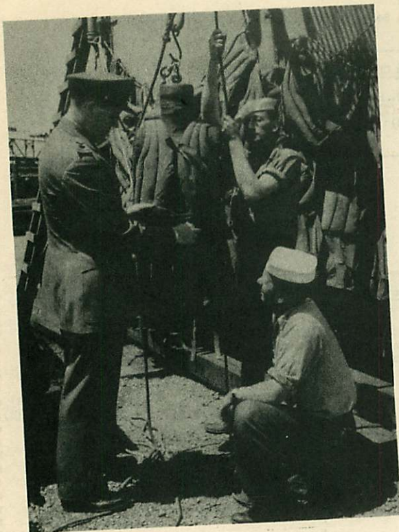
COAST GUARD OFFICER FITS A JACKET ON A STEEL DUMMY PREPARATORY TO ITS TRIP AROUND THE INTERIOR OF THE TANK
