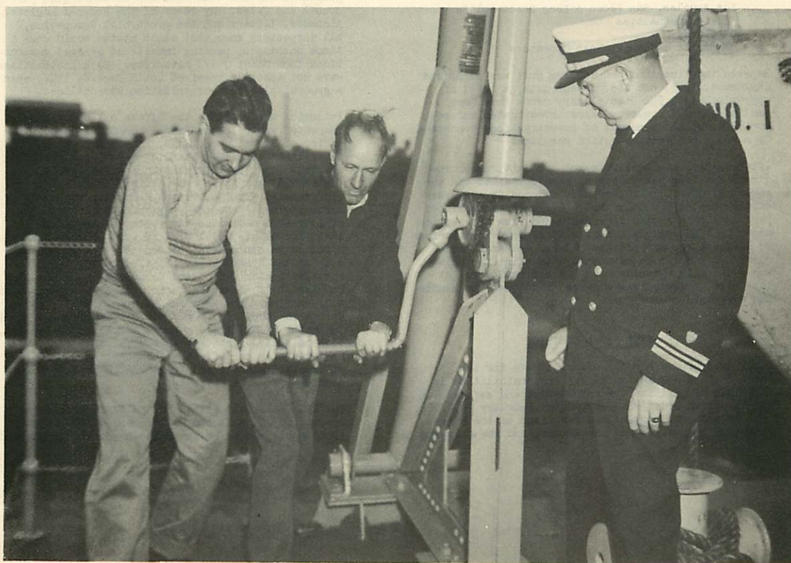
HAND HOISTING APPARATUS FOR THE PHOENIX LIFEBOATS GETS A WORKOUT FROM TWO DECK HANDS UNDER THE DIRECTION OF A COAST GUARD INSPECTOR
