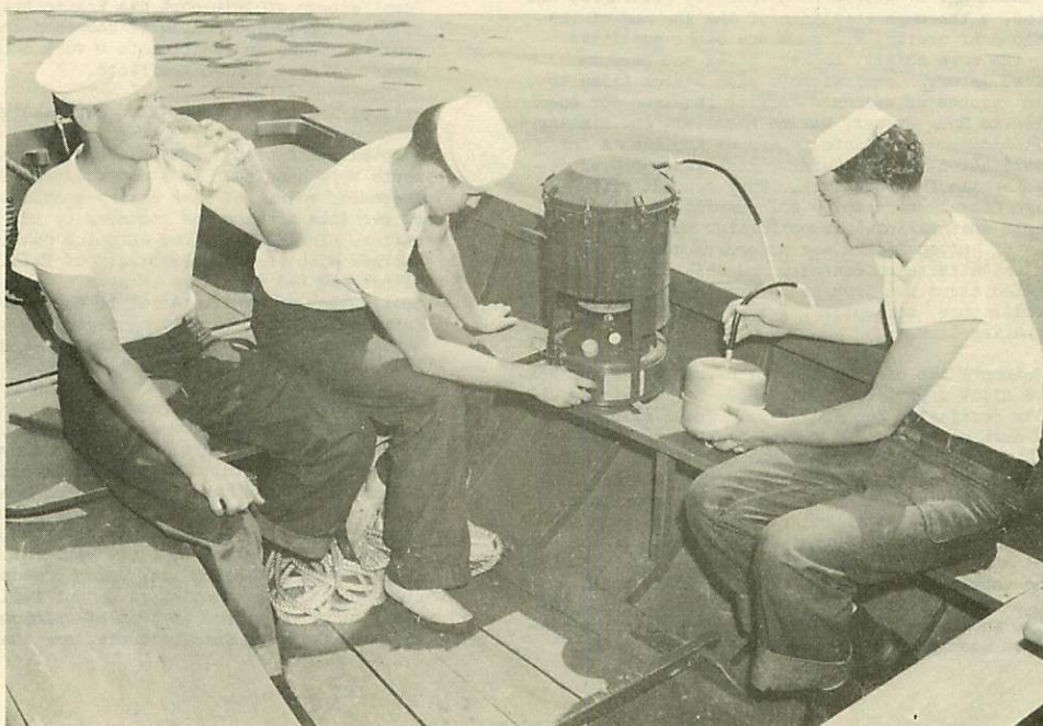
THIS PORTABLE COMBINATION WATER PURIFIER AND COOKING AND HEATING STOVE DESIGNED FOR USE IN LIFEBOATS IS SHOWN DURING TESTS BY U. S. COAST GUARDSMEN
