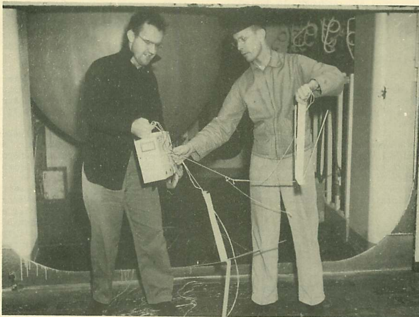
CIVILIAN WEATHER OBSERVERS PREPARING "RADIOSONDE" (INSTRUMENT WHICH MEASURES AIR TEMPERATURE, PRESSURE AND HUMIDITY AND TRANSMITS THIS INFORMATION TO RECEIVER ABOARD SHIP).
