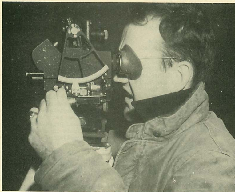
BALLOON IS TRACKED WITH THEODOLITE UNTIL ITS DISTANCE FROM THE SHIP IS GREAT ENOUGH SO THAT IT CAN BE PICKED UP BY SHIP'S RADAR
