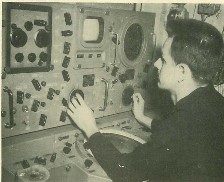
AFTER RADAR HAS CONTACT WITH THE BALLOON THEODOLITE TRACKING IS NO LONGER NECESSARY
