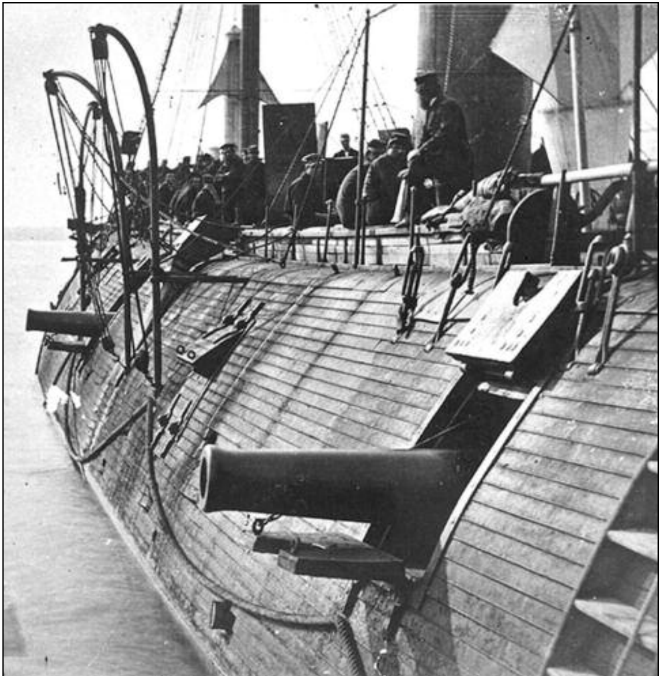
Figure 11. Matthew Brady photograph of the ironclad Galena after the Battle of Drewry's Bluff. A plugged shot hole is visible a little abaft the nearer 11-inch Dahlgren smoothbore, close to the waterline.
