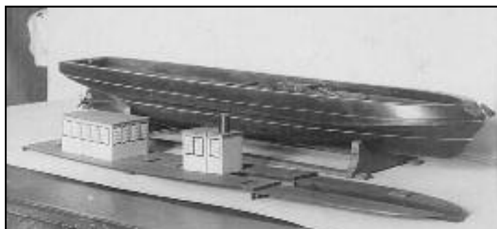
Figure 7. Contemporary model of the Civil War gunboat Naugatuck , Showing the armor belt and thick cedar bulwark.
