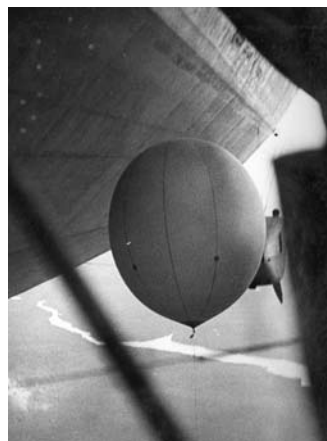
The expedition's state-of-the-art balloon sensor probe. The balloon dropped clear of the airship before ascending into the atmosphere to avoid getting caught in the zeppelin's motors
