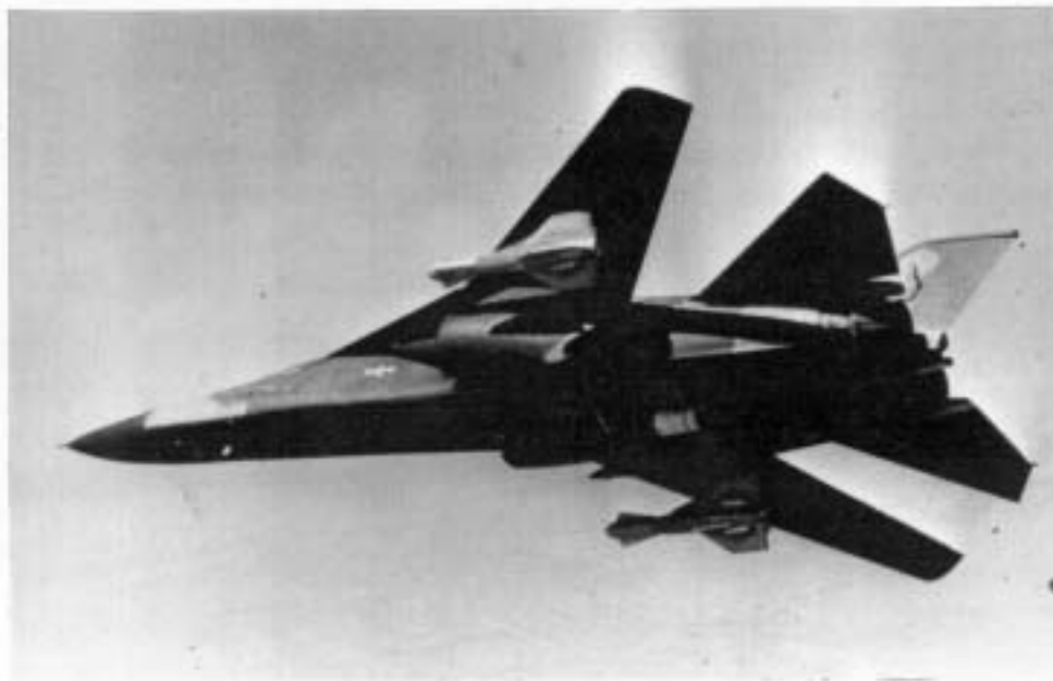
Fig 9. GBU-15s on F-111F (Armament Division, Eglin AFB)
