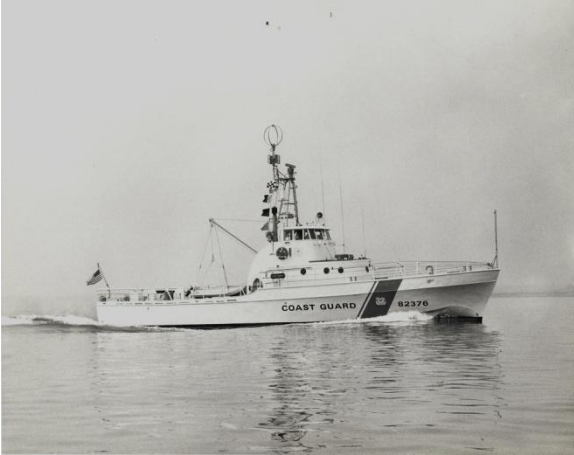
WPB-82376 Point Harris circa 1970 - RDF loop at masthead.
