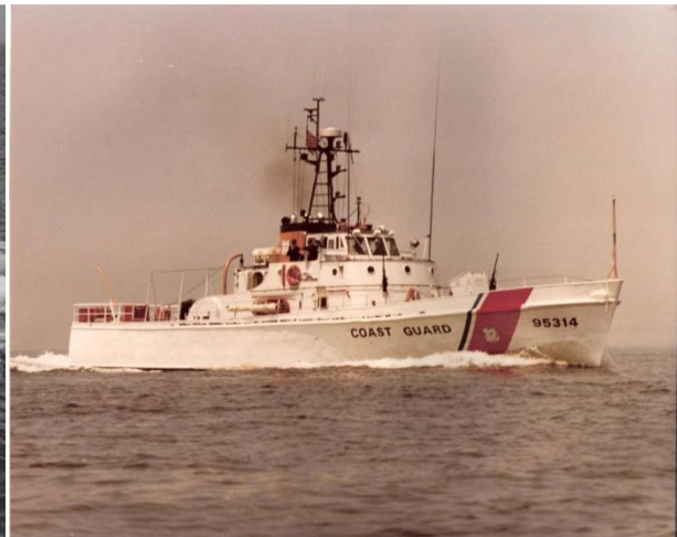
A pair of "B" class Capes: WPB-95312 Cape Knox and WPB-95314 Cape Fairweather . The former is shown circa 1970 mounting an over-under 50-cal m.g. above an 81-mm mortar (developed for use in Viet Nam). The latter mounts a lone 50-cal. m.g. circa 1980.
