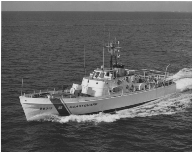
A pair of "B" class Capes: WPB-95312 Cape Knox and WPB-95314 Cape Fairweather . The former is shown circa 1970 mounting an over-under 50-cal m.g. above an 81-mm mortar (developed for use in Viet Nam). The latter mounts a lone 50-cal. m.g. circa 1980.
