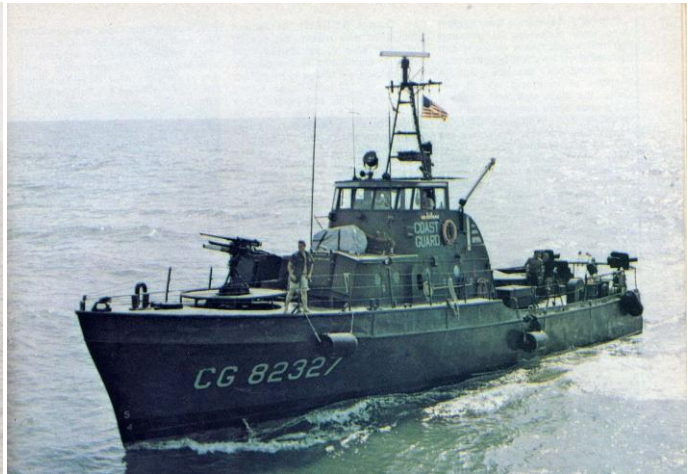
Two sisters from Squadron One in Viet Nam War Paint WPB-82323 Point Grace and 82327 Point Banks circa 1968. Both mount the usual over-under 50-cal m.g. and 81-mm mortar combo in the bow, while additional 50's are mounted aft.
