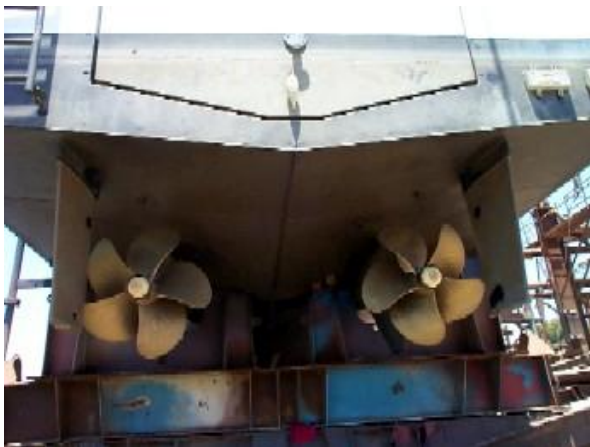
Haddock's stern showing 5-bladed props
