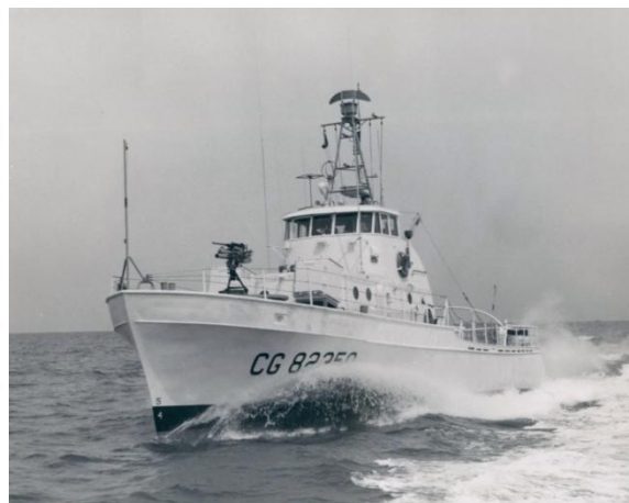
WPB-82340 Pt. Batan & 95320 Cape Starr fight barge fire in 1980's. WPB-87350 Pt. Franklin circa 1963 with over-under m.g. & 81-mm mortar forward.
