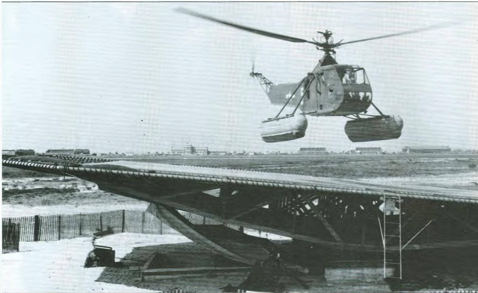
**Above:** *The Mal de Mer, or "sea sick," was built by the Coast Guard Special Services Division to simulate the movement of a ship's deck when a helicopter was about to land on it.*
