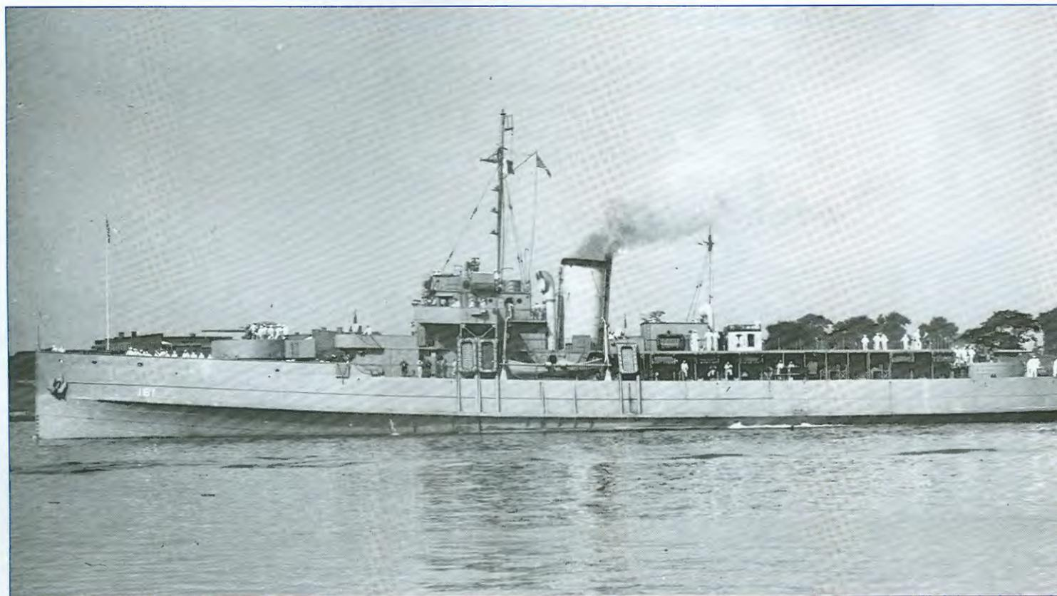
several depth charge arrangements. After conversion, the 37-year-old ship had the double distinction of being the first turbine-driven ship built in the United States and the first helicopter carrier.
