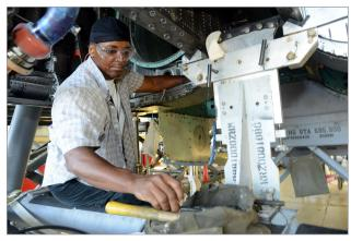
U.S. Air Force structural repair technician, installs fasteners into the newly replaced 626 bulkhead of an F-15C
