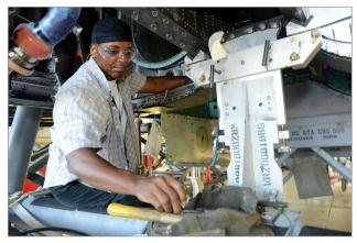
U.S. Air Force structural repair technician, installs fasteners into the newly replaced 626 bulkhead of an F-15C Source: Air Force
