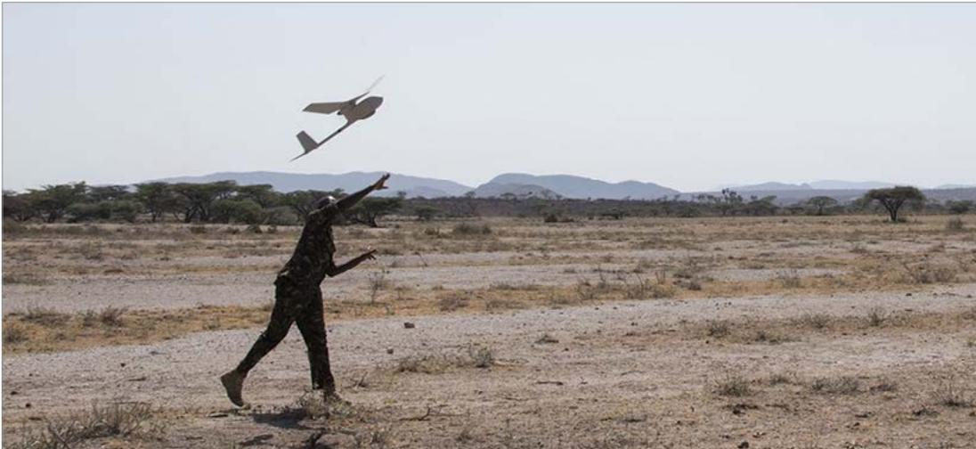
Figure 5. Kenyan Defense Forces Soldier Launches Raven Unmanned Aerial Vehicle (UAV)
