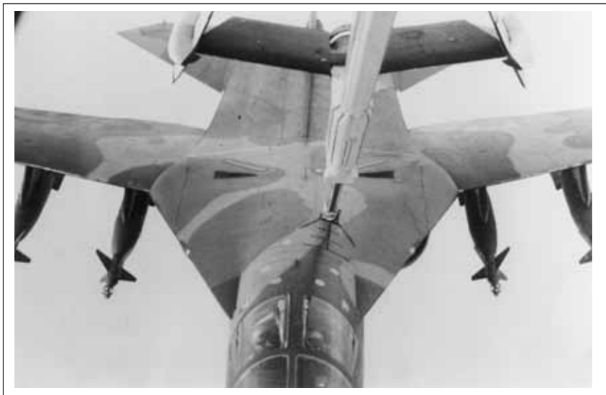
With only the UK offering use of its bases, US aircraft faced a long flight to Libya. The round trip required eight to 12 in-flight refuelings for each airplane—this one, from Karma Flight, armed with 2,000-pound laser-guided bombs.
