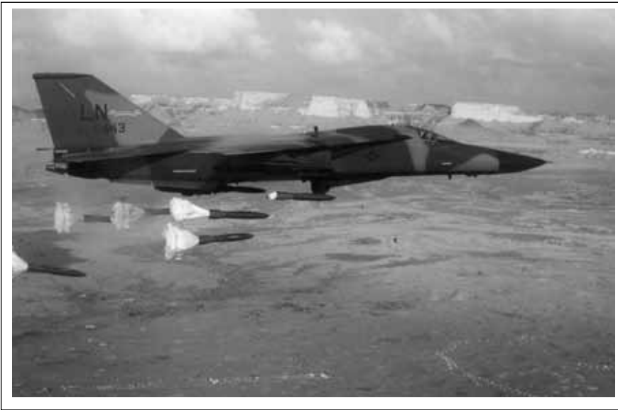
Puffy and Lujac attack elements, armed with Mk 82 Snakeye parachute-retarded 500-pound bombs like these, struck the Tripoli airport. The operation led to F-111 changes that would make the aircraft invaluable in the Gulf War.
