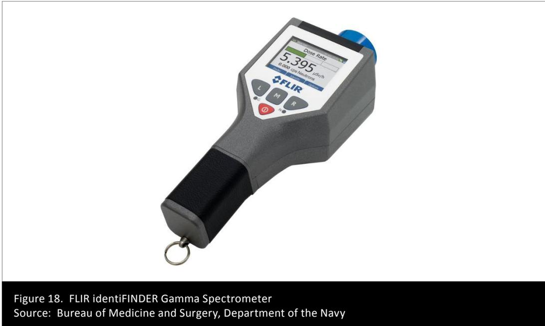
Figure 18. FLIR identiFINDER Gamma Spectrometer
