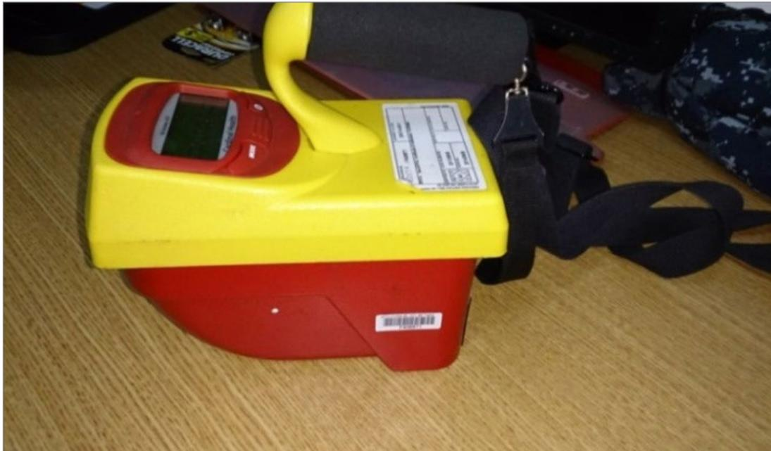
Figure 15. FLUKE 451P ionization chamber
