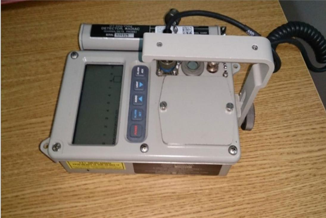
Figure 16. SAIC IM-265/PDQ with DT 680 Beta-Gamma probe
