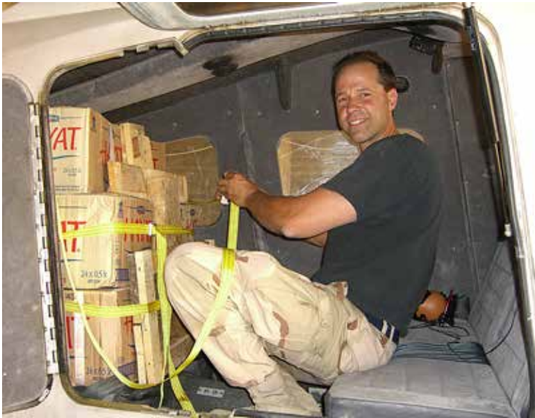
Dean van Oosterhout setting up for a center-of-gravity test in the CA-7 aircraft during Phase I in Kirkuk, October 11, 2005. (Photo courtesy of Dean van Oosterhout)
