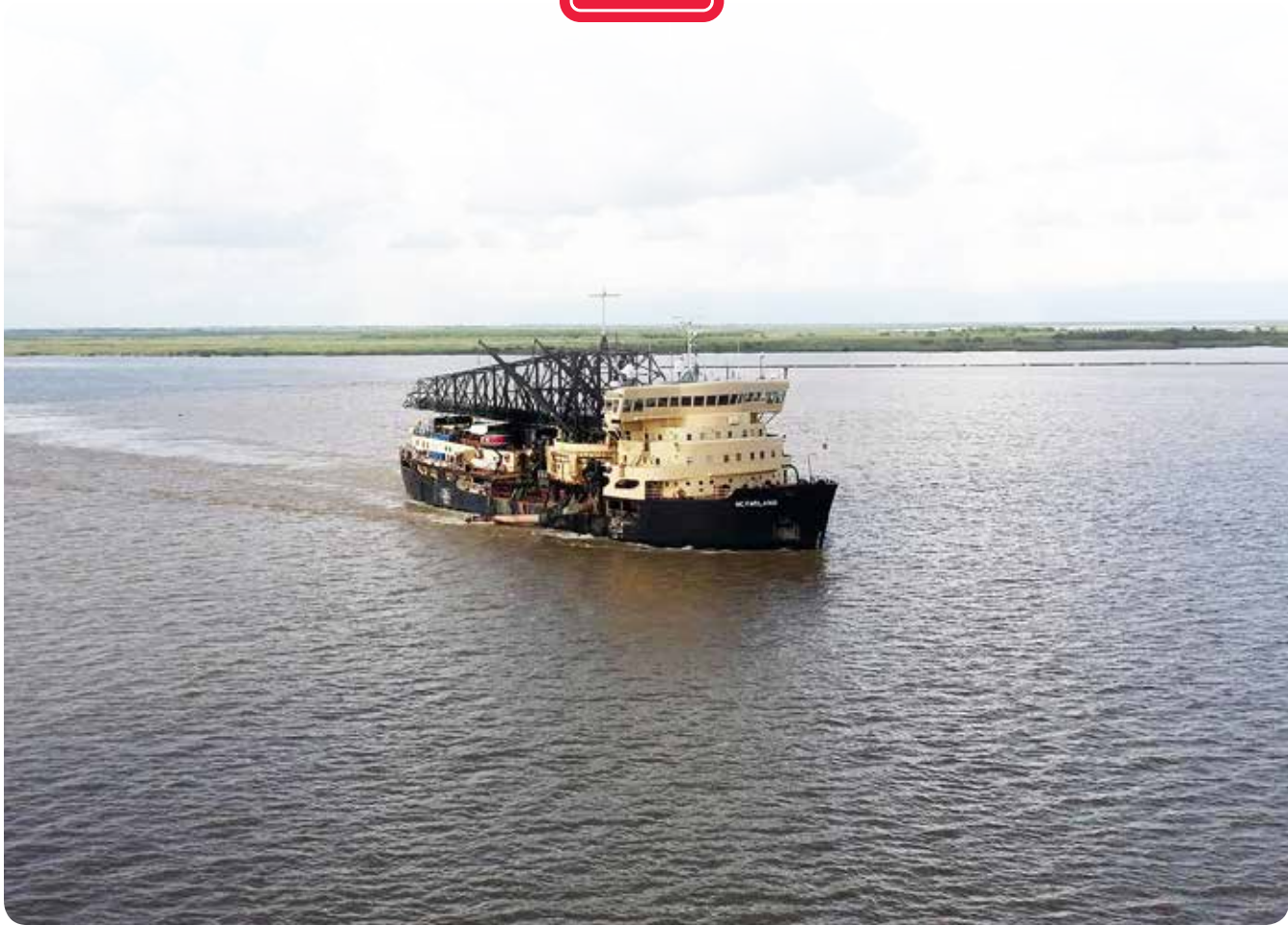
The McFarland, a deep-draft hopper dredge owned and operated by USACE Philadelphia District, conducts urgent dredging for 62 days on the Southwest Pass of the Mississippi River. (Photo courtesy of U.S. Army Corps of Engineers)
