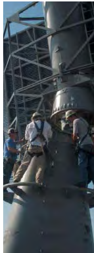
Placing the SPS-48 air search radar on the USS Abraham Lincoln while undergoing a refueling complex overhaul (RCOH) at Newport News Shipbuilding. (U.S. Navy photo by Mass Communication Specialist 3rd Class Ryan L. Wampler/Released)
