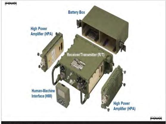
Figure 2. (FOUC) Manpack radio Source: (COUO) Program Executive Office for Command, Control, Communications-Tactical
