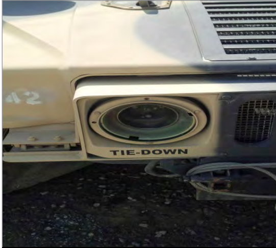
Figure 7. HMMWV with missing headlights Source: DoD IG
