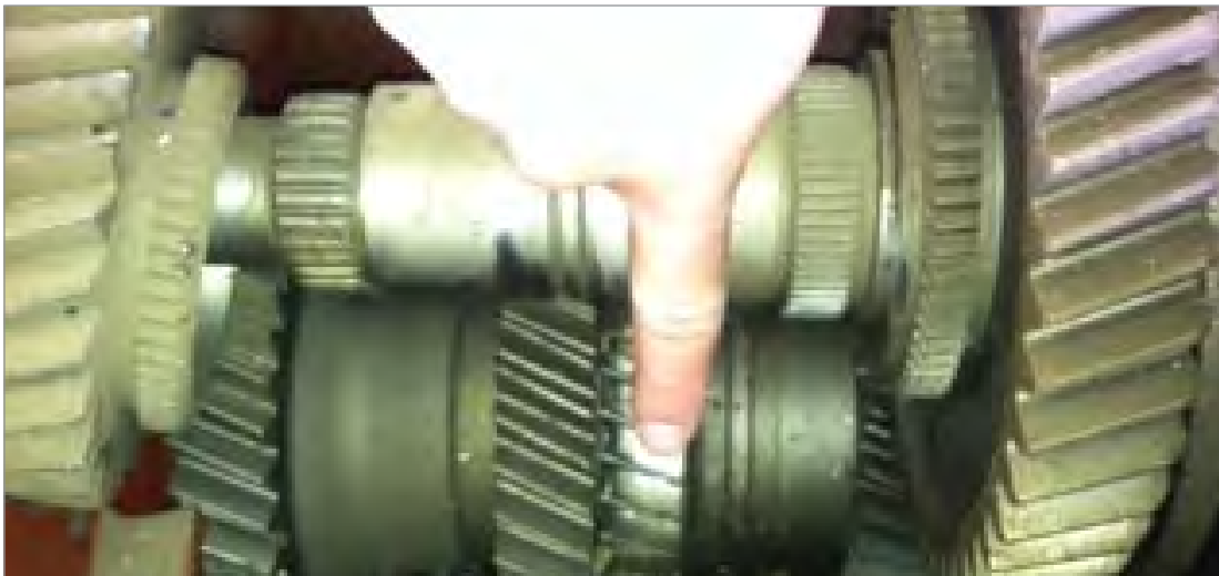
Figure 6. Gearbox with the gears stripped Source: DoD IG
