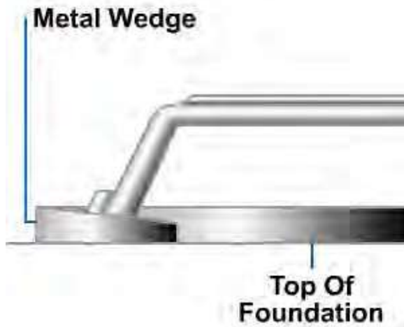
Figure 7-25 — Wedging a base plate.
