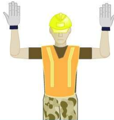
Manuever Forward Slowly When maneuvering in close quarters or to move a foot or two at a time.
