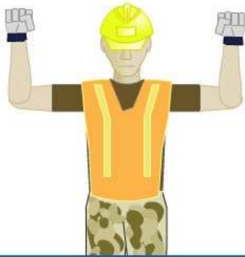
Emergency Stop Stop all motion as quickly as possible.
