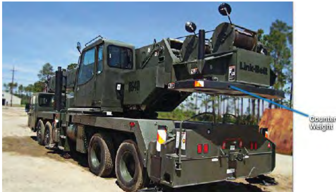
Figure 21-22 – Counterweight on a truck-mounted telescopic boom.
