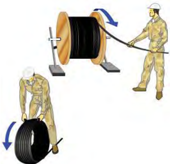
Figure 22-20 — Unreeling wire rope and uncoiling wire rope.
