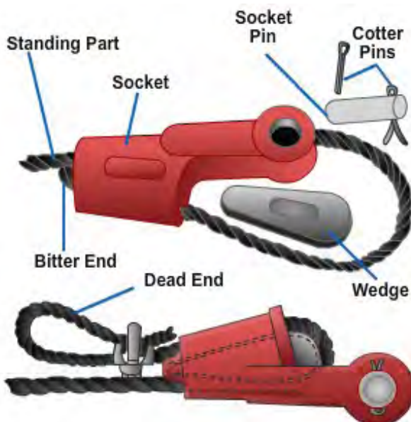
Figure 22-27 – Wedge socket. 22-30
