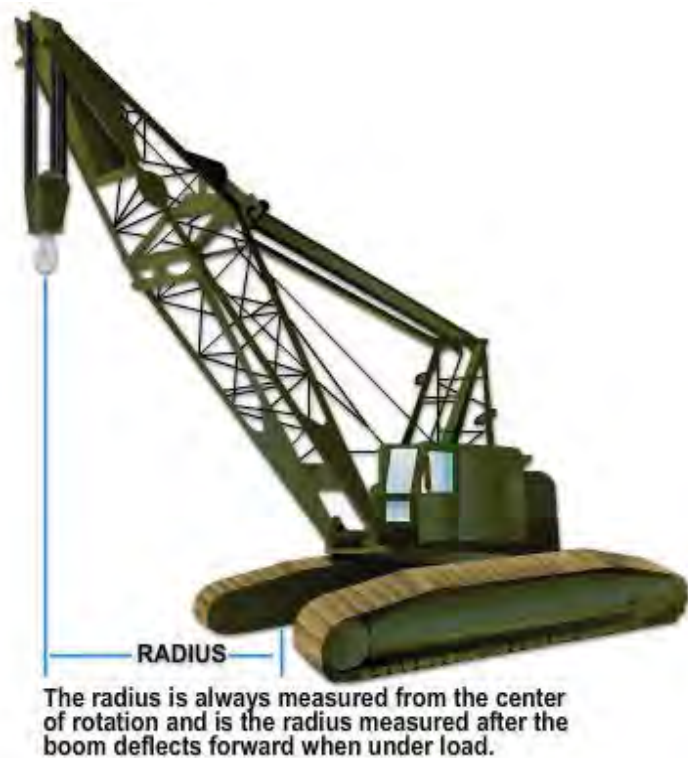
Figure 21-3 – Crane radius measurement.
