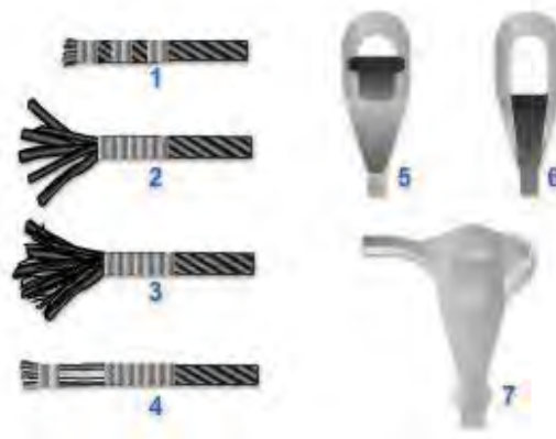
Figure 22-28 — Speltering a socket.
