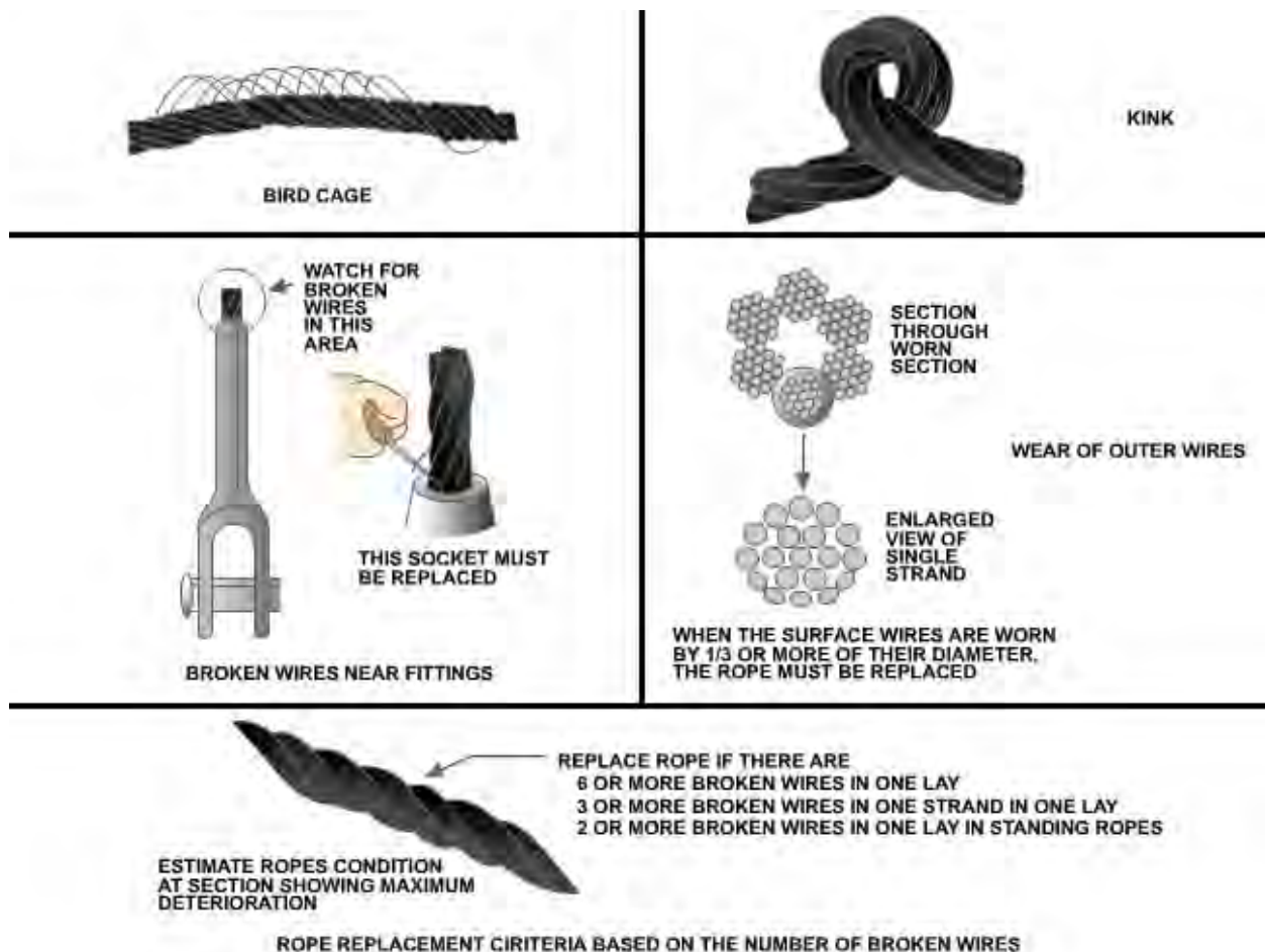
Figure 21-65 – Common wire rope defects.
