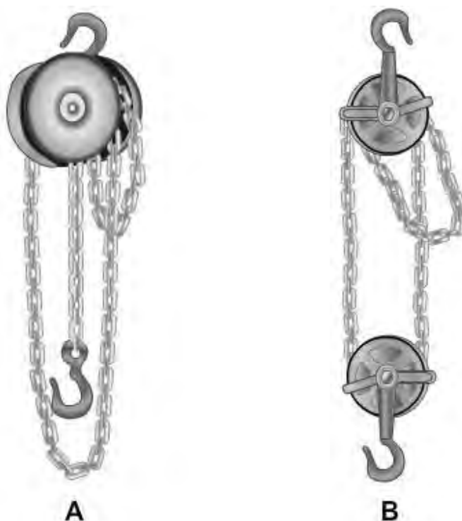
Figure 22-47 — View A: Spur gear chain hoist; View B: Differential chain hoist.
