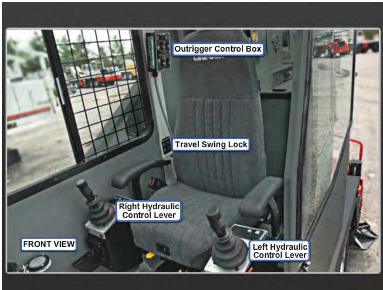
Figure 21-25 – Controls on a telescopic boom truck-mounted crane.
