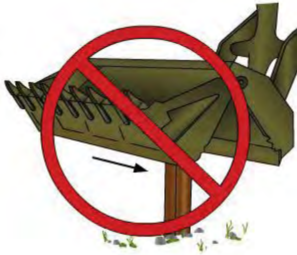
Figure 13-38 – Breaking off an object by side loading the clamshell.
