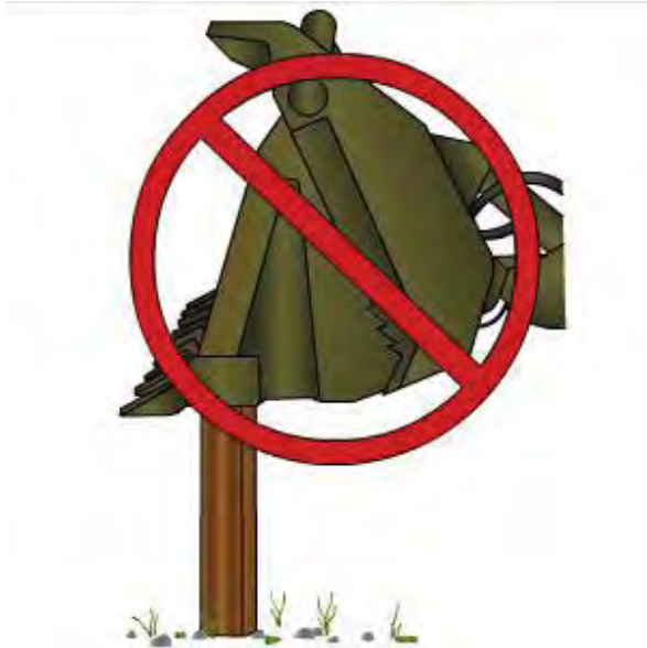
Figure 13-42 – Using the bottom of the clamshell as a pile driver.
