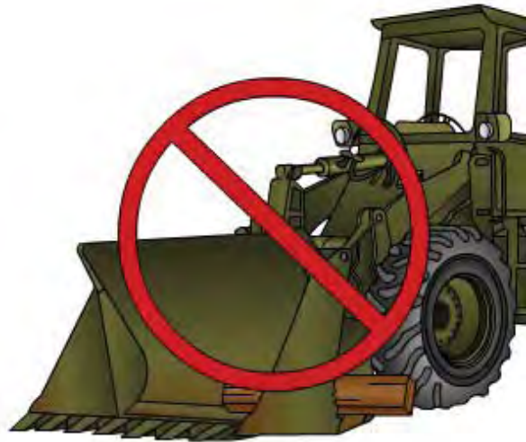
Figure 13-39 – Clamping an object on only one side of the clamshell.
