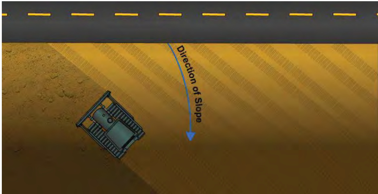
Figure 19-32 – Finishing a side slope by working diagonally.
