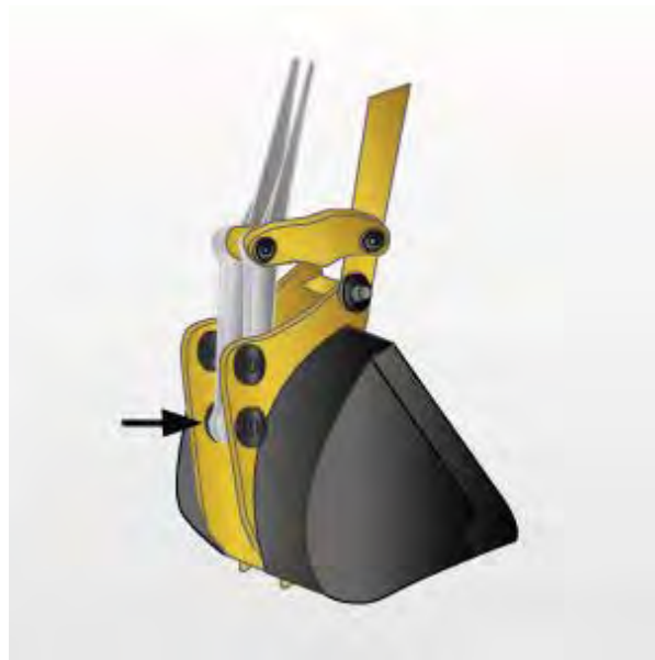
Figure 14-8 – Position for digging deep vertical holes.
