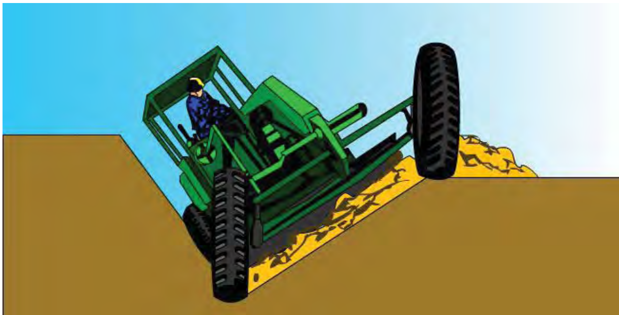
Figure 17-12 – Wheel lean on a ditch slope
