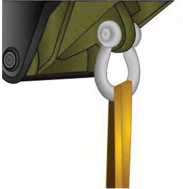
Figure 14-24 – Rigging a sling to the bucket.
