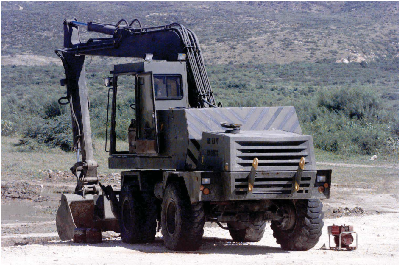
Figure 15-3 – Truck-mounted excavator with a standard hydraulic boom.
