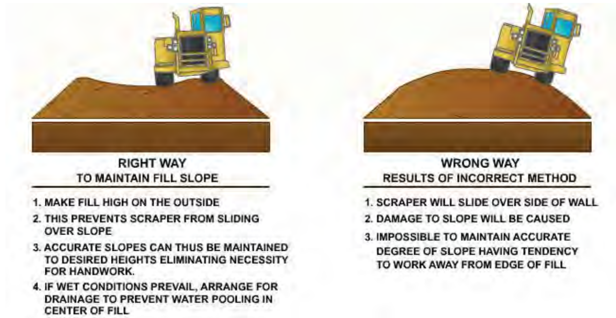
Figure 18-21 – Proper placement to fill material.
