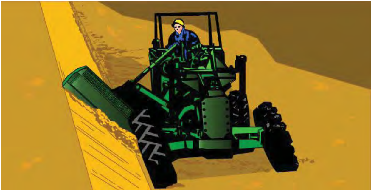
Figure 17-13 – Wheel Lean on high bank-cutting operations.
