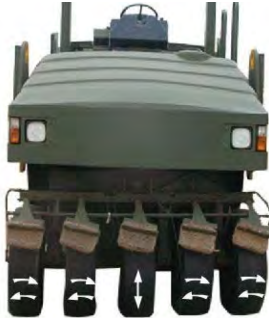
Figure 20-3 – Action of a pneumatic-tired roller.
