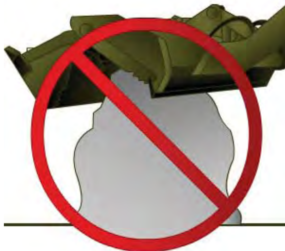
Figure 13-44 – Attempting to pickup objects too large for the clamshell.
