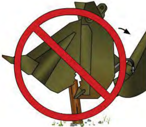
Figure 13-36 – Removing buried objects using the clamshell by rolling back the bucket.
