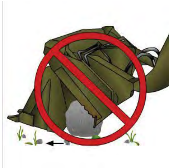
Figure 13-43 – Attempting to load material with an object caught in the clamshell.
