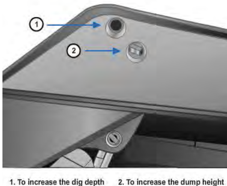
Figure 15-7 – Boom depth-height adjustment.
