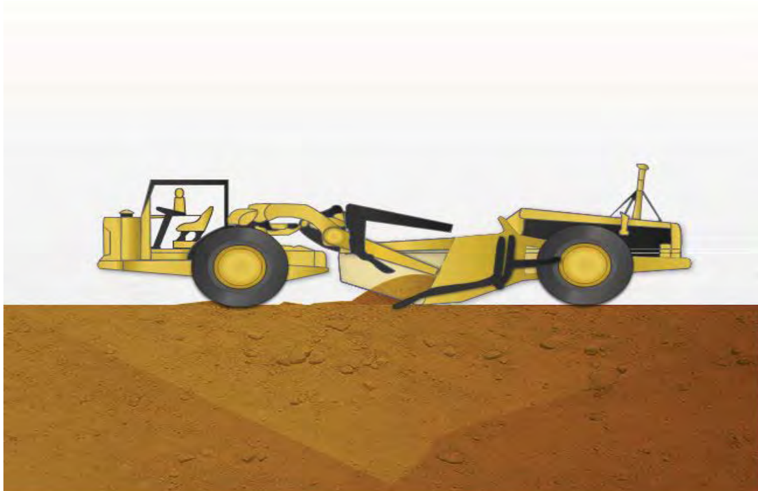
Figure 18-12 – Entering the cut.
