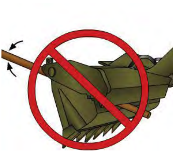
Figure 13-40 – Clamping an object and using it as a battering ram.
