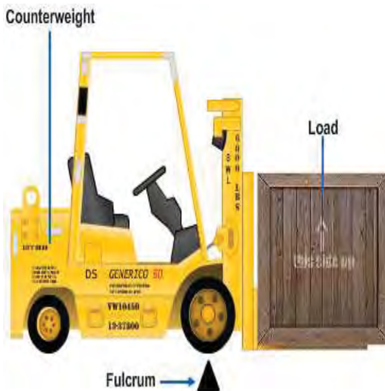
Figure 12-32 – Forklift operates as a fulcrum.
