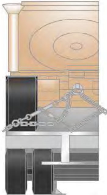
Figure 10-56 – Crossed chains for inadequate chain length with the same side pattern.
