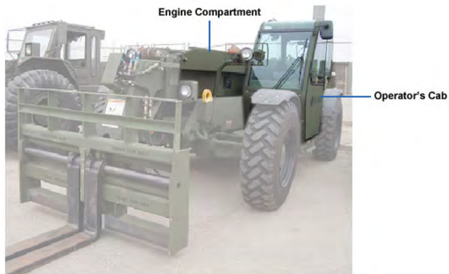
Figure 12-16 – 11K MMV Operator's Cab and engine compartment.
