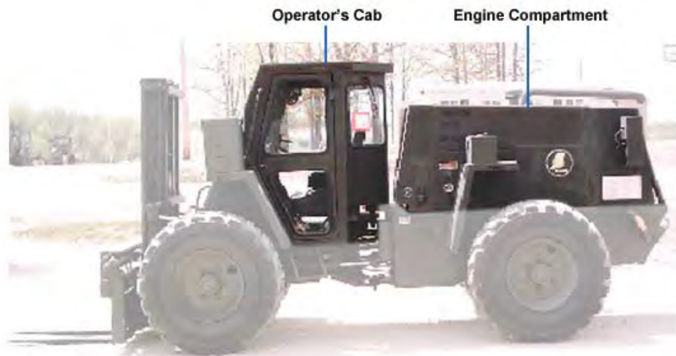
Figure 12-8 – 4K RT forklift operator's cab and engine compartment.
