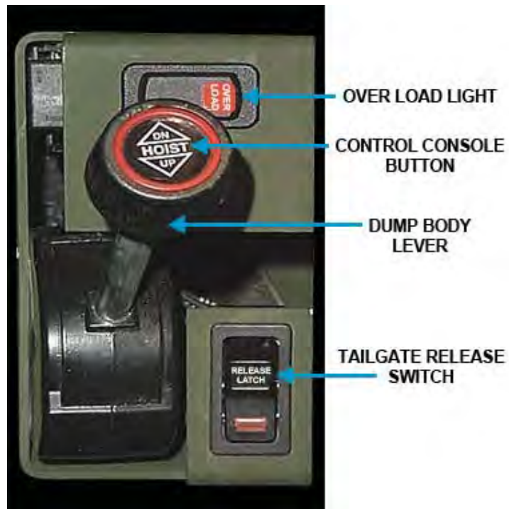
Figure 8-8 – Dump body controls.
