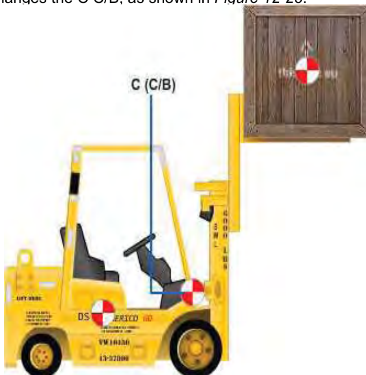
Figure 12-28 – Forklift combined center of balance with a load.
