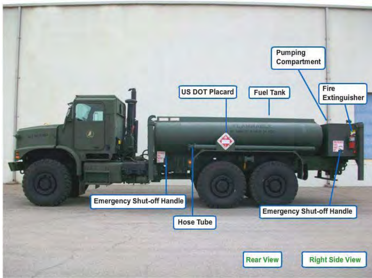
Figure 9-1 – Major components of a fuel truck.
