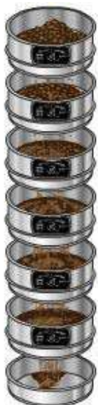
Figure 16-2 – Typical sieves used for particle size identification.
