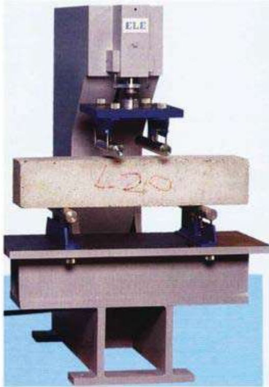
Figure 16-52 - Example of flexural strength test.
