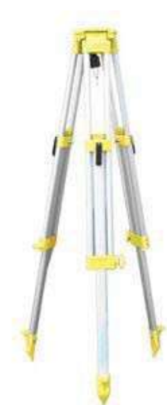
Figure 17-4 — Typical surveyor's tripod.
