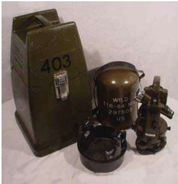
Figure 17-2 — Examples of typical instrument cases.
