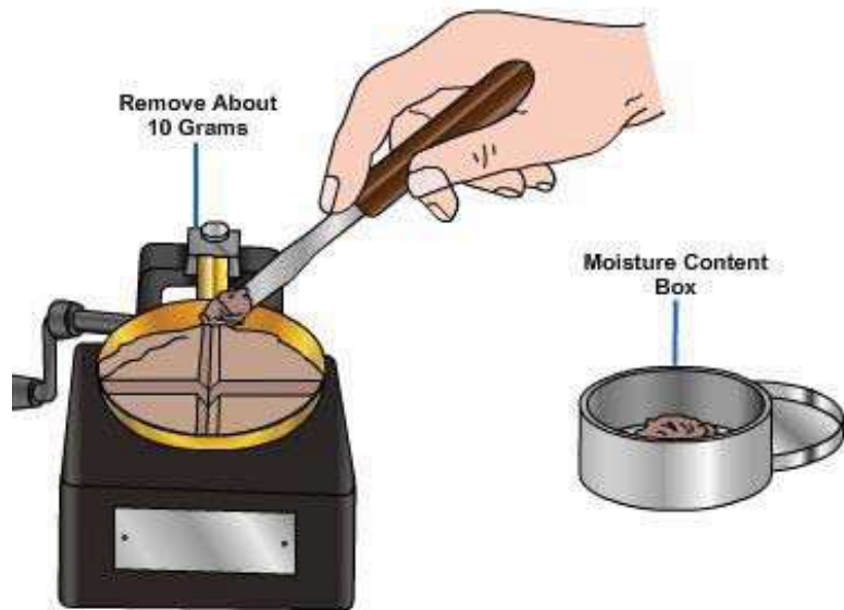
Figure 16-47 - Example of removing sample for moisture determination.
