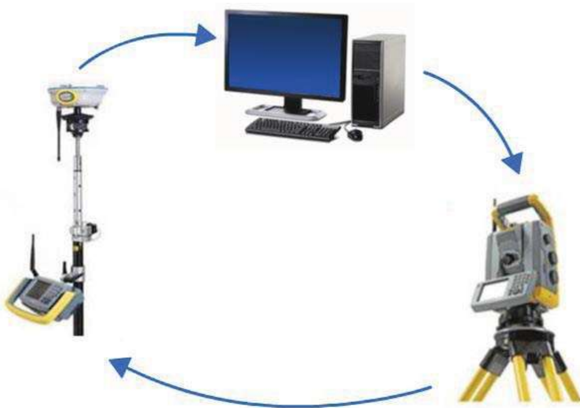
Figure 17-18 – Data flow using Trimble® 5600 Total Station.
