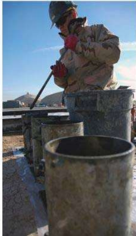
Figure 16-57 - Seabee making typical concrete cylinder molds.
