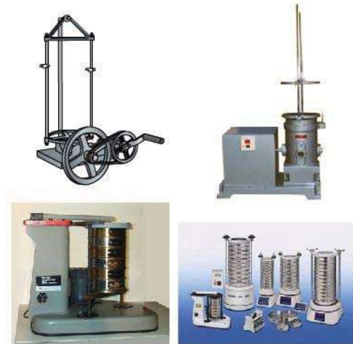
Figure 16-32 – Example of types of sieve shakers.
