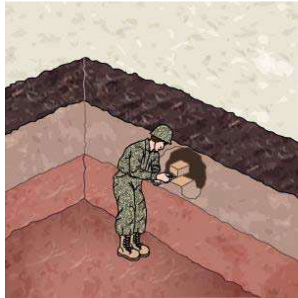
Figure 16-17 – Example of taking a chunk sample from a vertical surface.
