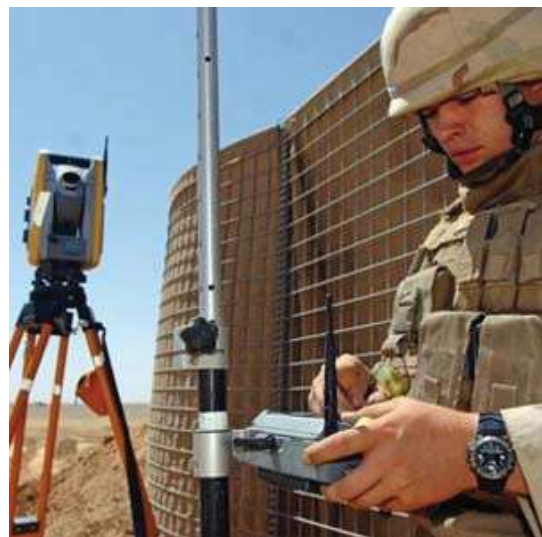
Figure 17-19 – Trimble®/Geodimeter Total Station with ACU.
