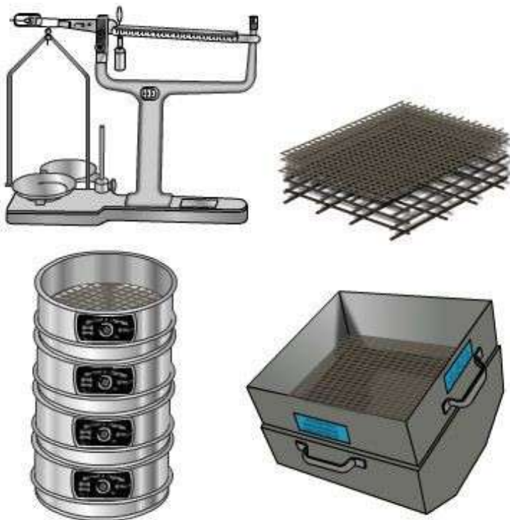
Figure 16-31 - Typical sieve set apparatus.
