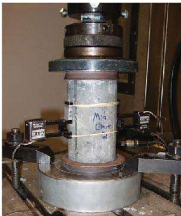
Figure 16-51 - Example of concrete cylinder compression test.
