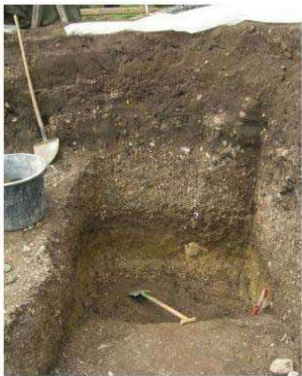
Figure 16-6 – Example of a soil sampling test pit.
