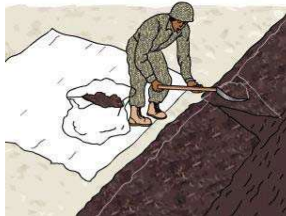
Figure 16-13 – Example of taking a composite soil sample from a windrow.
