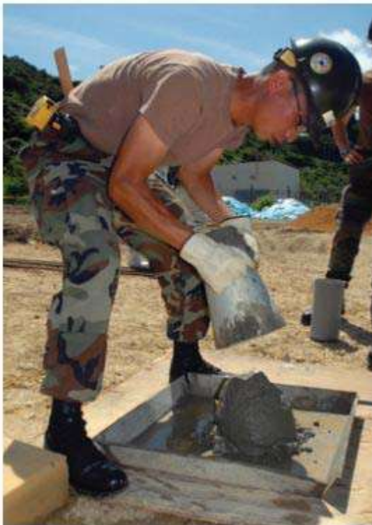
Figure 16-55 - Seabee performing slump test.
