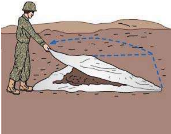
Figure 16-26 – Example of quartering a soil sample of 25-100 pounds.
