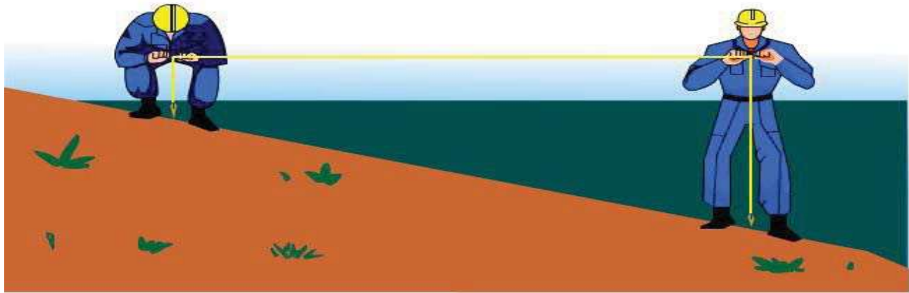
Figure 13-11 – Horizontal chaining using plumb bobs.
