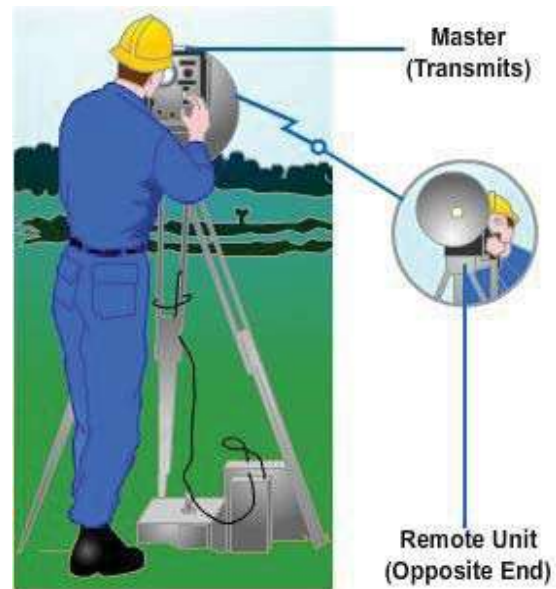
Figure 13-21 – Setting a microwave distance-measuring unit.
