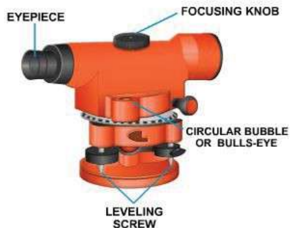
Figure 12-11 - An automatic level.
