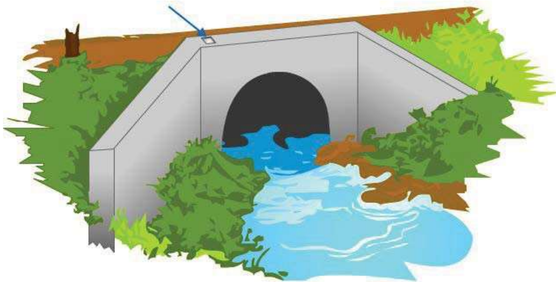
Figure 15-3 - Benchmarks located on concrete structure.
