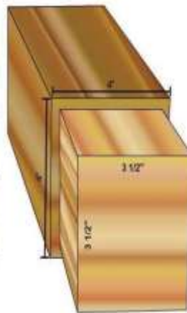
Figure 7-2 — Nominal and dressed sizes of lumber.
