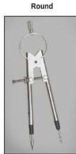
Figure 3-22 - Shapes of compasses and dividers.
