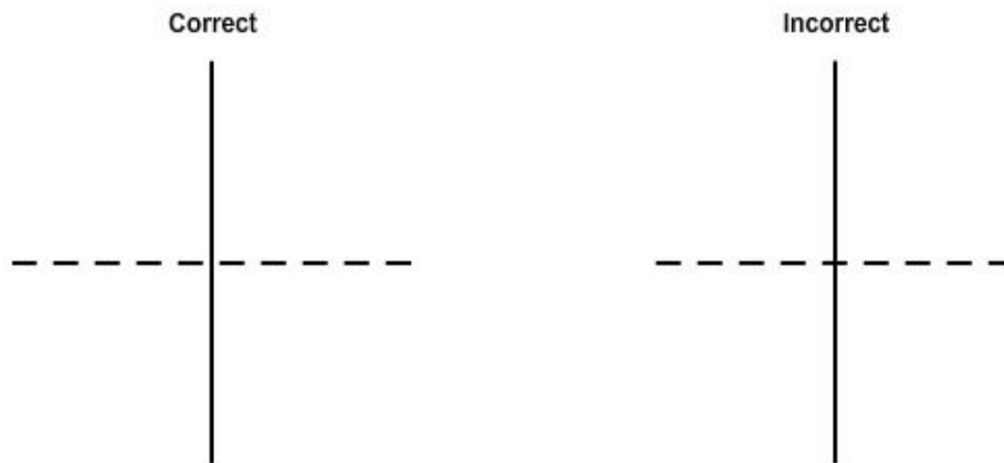
Figure 4-33 - Correct and incorrect procedures for drawing a hidden edge line that intersects a visible edge line.
