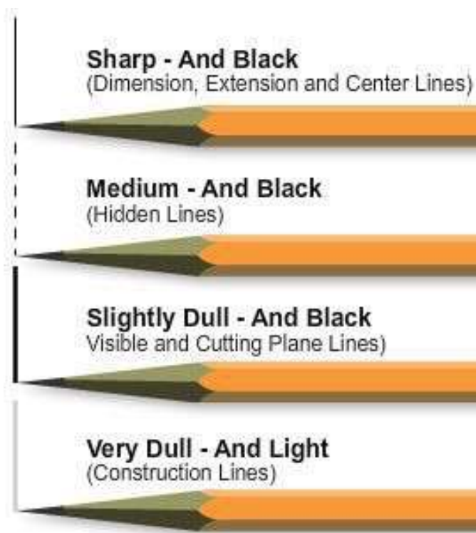
Figure 6-58 - Line conventions drawn with various types of pencil points.
