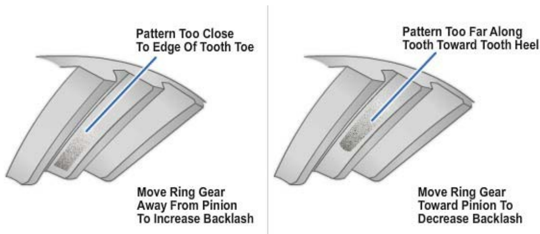
Figure 8-101 - Two incorrect patterns when adjusting backlash.
