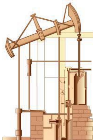
Figure 4-3 – 1769-James Watt's improved steam engine powered the industrial revolution.
