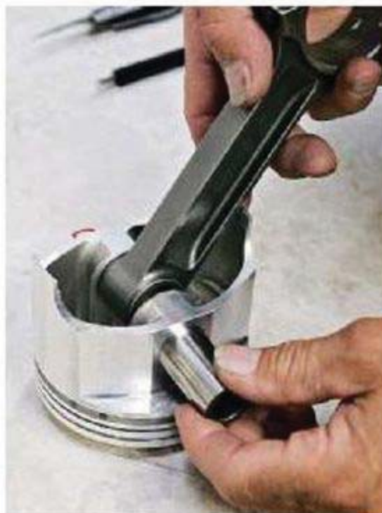
Figure 4-33 - A free-floating piston.
