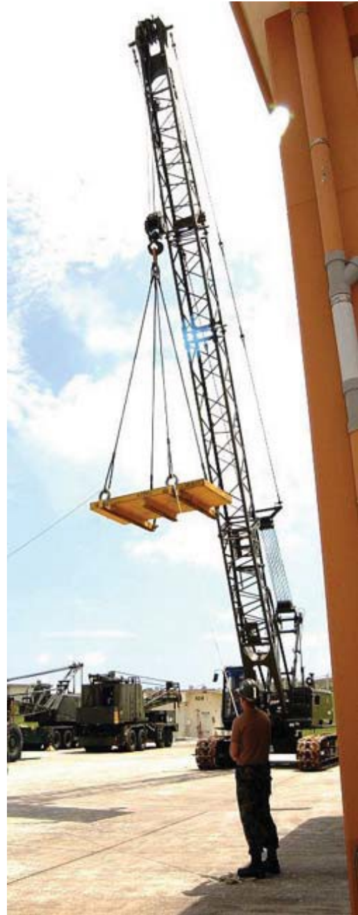
Figure 3-13 – A 50-ton LinkBelt lattice boom crane being certified using an 11,850-pound weight in Okinawa.
