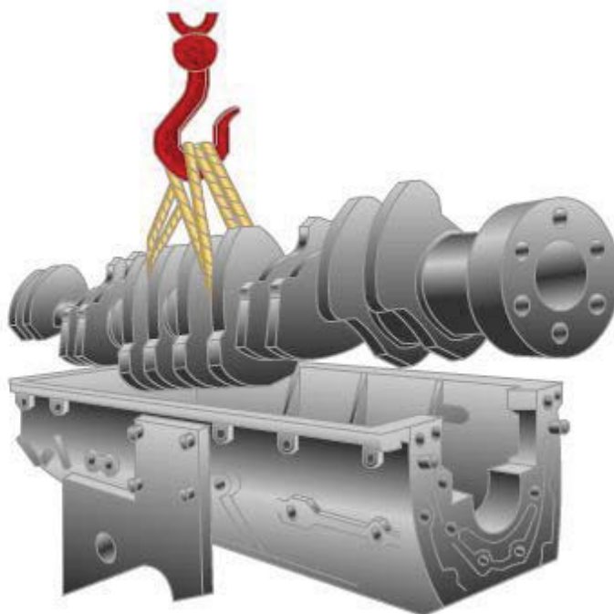
Figure 4-26 - Removing the crankshaft with a hoist.
