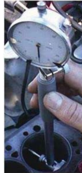
Figure 4-30 – Dial bore gauge.
