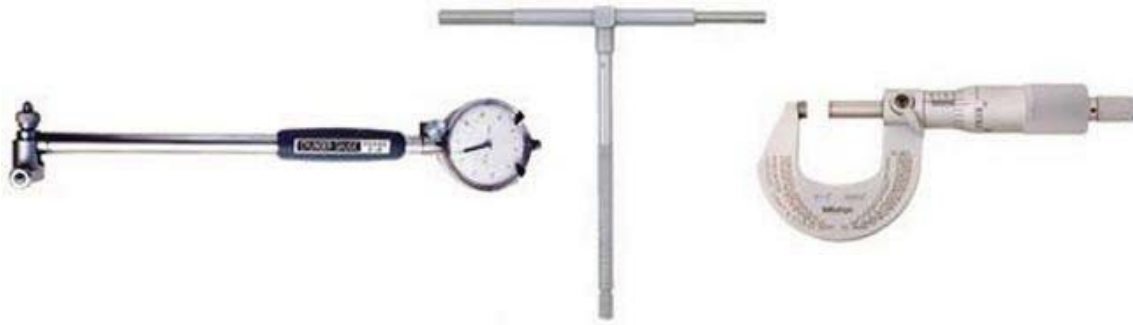
Figure 4-24 - Tools used for camshaft bearing replacement
