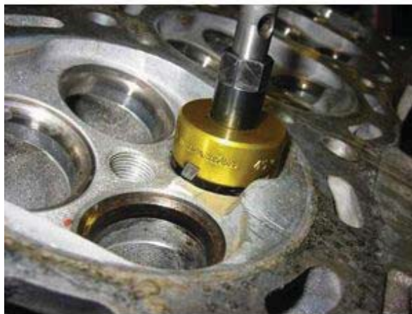
Figure 4-20 – Valve seat grinding.
