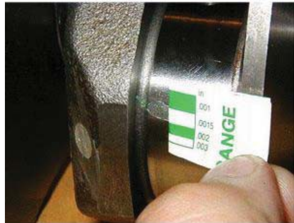
Figure 4-28 – Using Plastigage to check bearing clearance.
