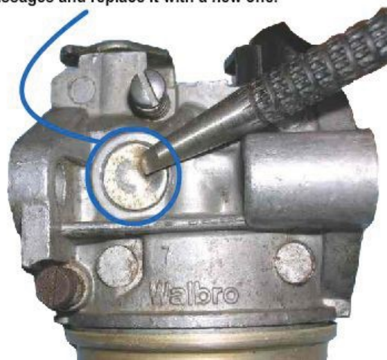
Figure 5-43- Remove Welch plug to check clogged passages.
