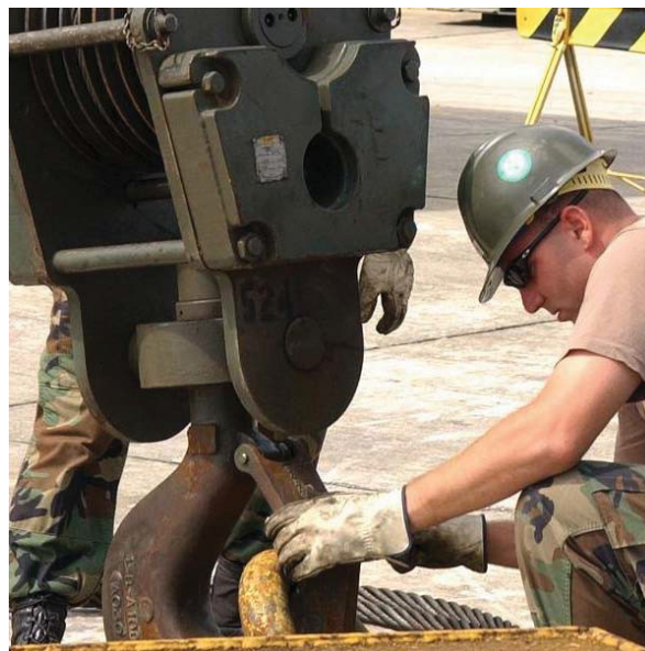
Figure 2-7 - Construction mechanics hooking the hoist to a calibrating weight to certify the crane's computer.
