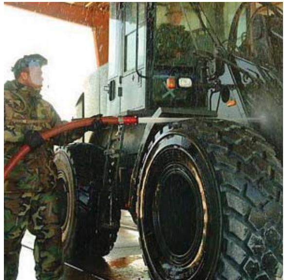
Figure 2-20 - Washing equipment to remove all grease and dirt and to detect fluid leaks prior to loading on aircraft.
