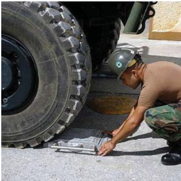
Figure 2-21 – Positioning scales to obtain axle weight of a wheeled vehicle for an air embarkation exercise.
