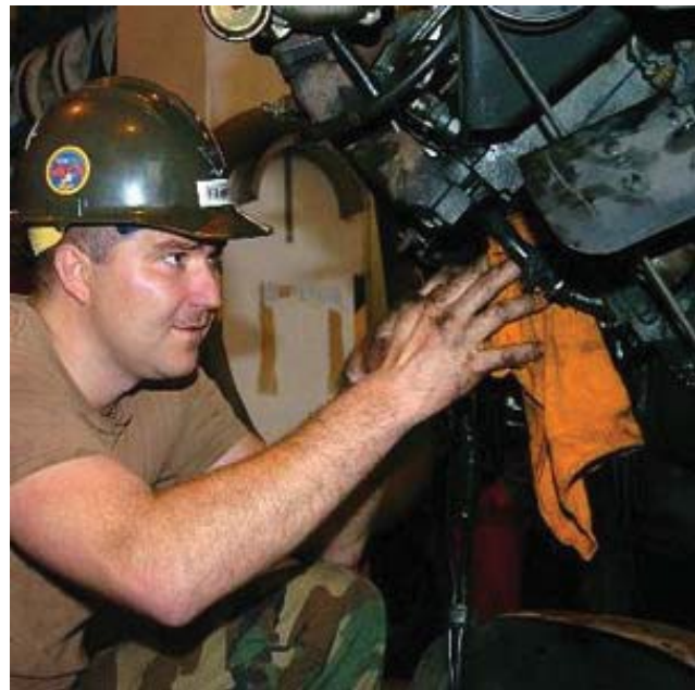
Figure 2-15 - Construction mechanic checks for leaks on an engine before reinstalling it back into a Chevy Coupe V truck.
