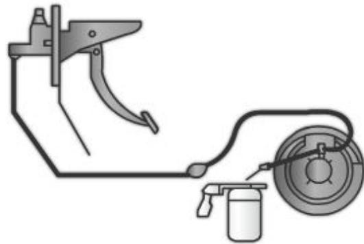
**Figure 13-24 — Vacuum bleeding a brake system.**
