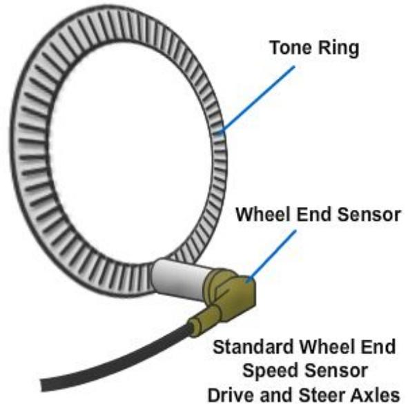
**Figure 13-44 — Wheel speed sensor.**
