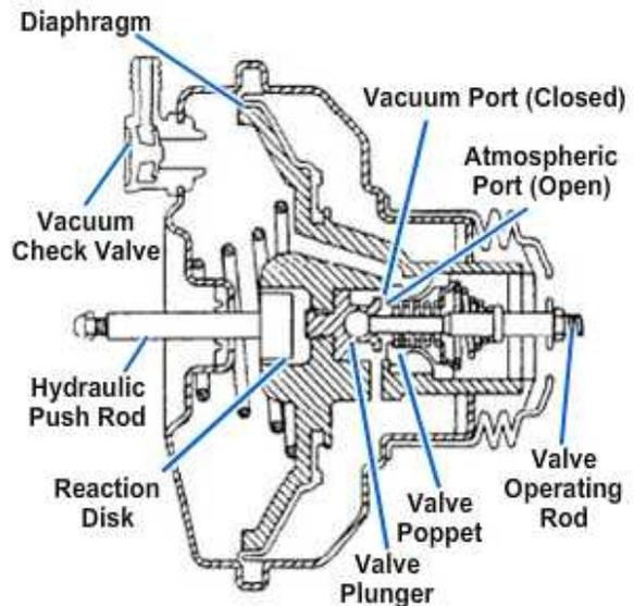
**Figure 13-15 — Vacuum brake booster.**
