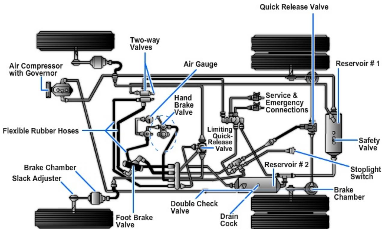
**Figure 13-26 — Typical air brake system.**
