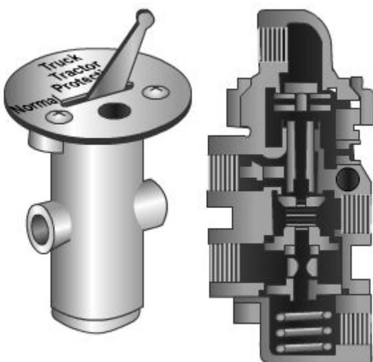
**Figure 13-36 — Tractor protection valve and switch.**
