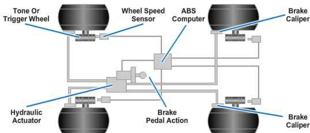
Figure 13-14 — Basic antilock brake system.
