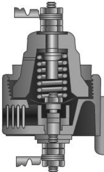
**Figure 13-42 — Low-pressure warning indicator.**
