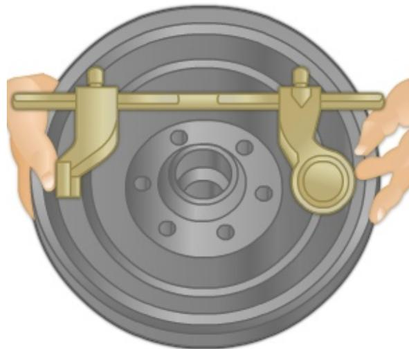
**Figure 13-21 — Using a drum micrometer to measure a drum.**
