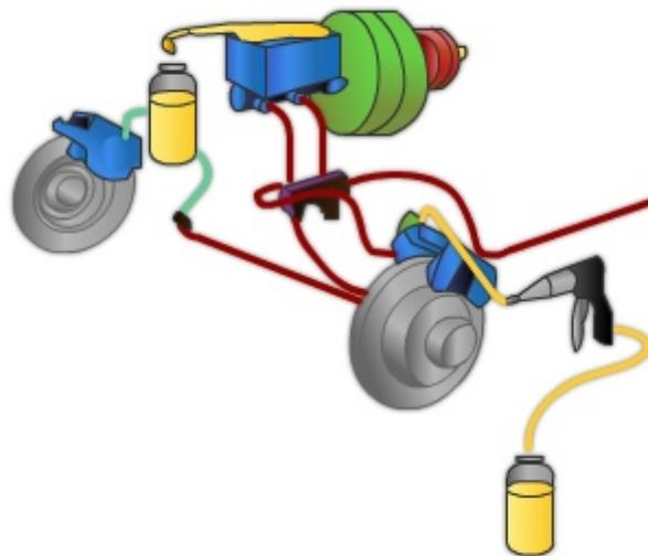
**Figure 13-25 — Force bleeding a brake system.**
