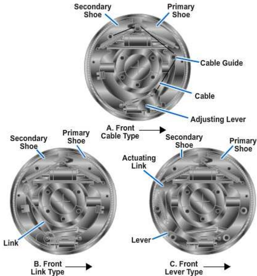
**Figure 13-9 — Self-adjusting mechanisms.**
