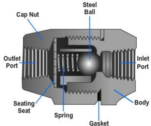
**Figure 13-39 — Ball-type single check valve.**
