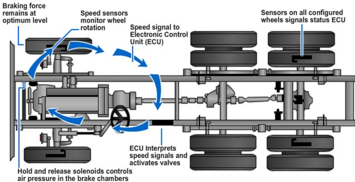
**Figure 13-45 — Air brake antilock brake system.**
