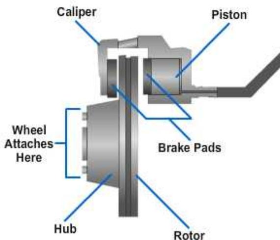
**Figure 13-11 — Disc brake assembly.**
