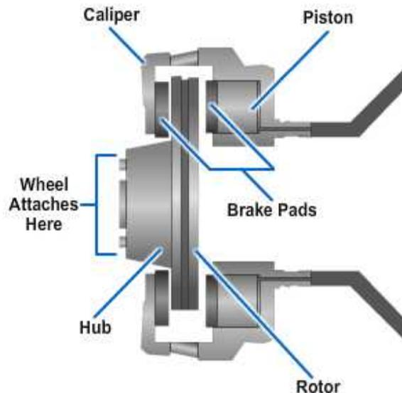
**Figure 13-13 — Fixed caliper.**
