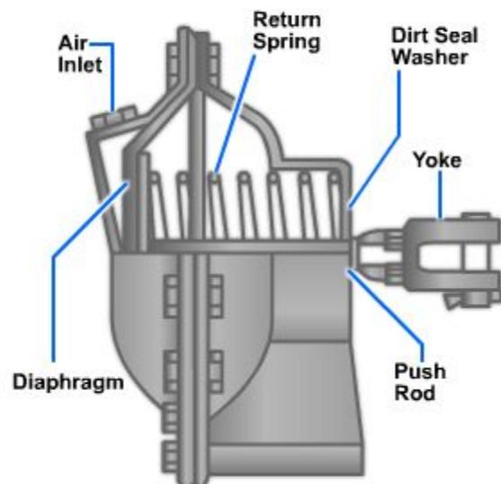
**Figure 13-32 — Air brake chamber.**
