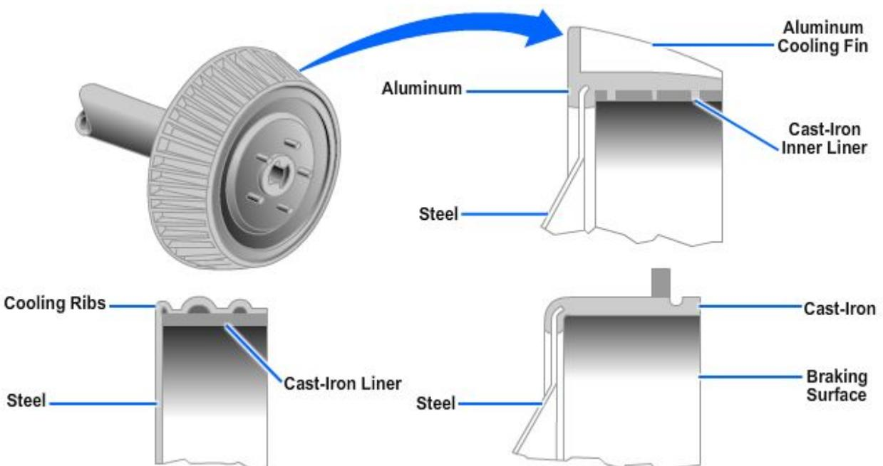
**Figure 13-8 — Brake drum construction.**
