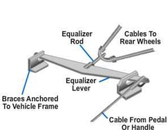
**Figure 13-19 — Equalizer linkage.**
