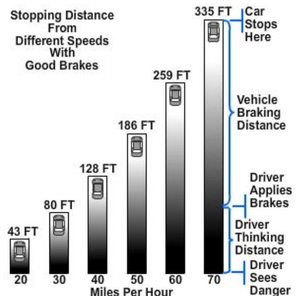
**Figure 13-1 — Total vehicle stopping distance of an average vehicle.**
