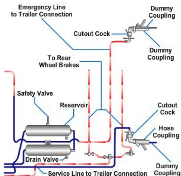
**Figure 13-37 — Tractor protection valve piping.**
