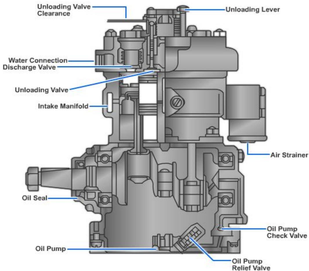
**Figure 13-27 — Typical two cylinder reciprocal air compressor.**
