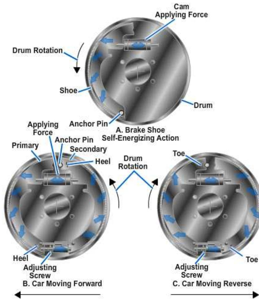
**Figure 13-10 — Self-energizing and servo action.**
