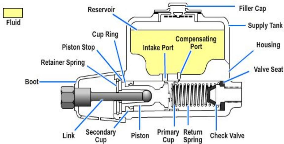
**Figure 13-2 — Cutaway view of a single master cylinder.**
