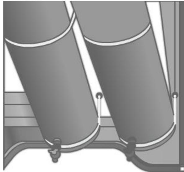
**Figure 13-31 — Air reservoir with an air drain valve.**
