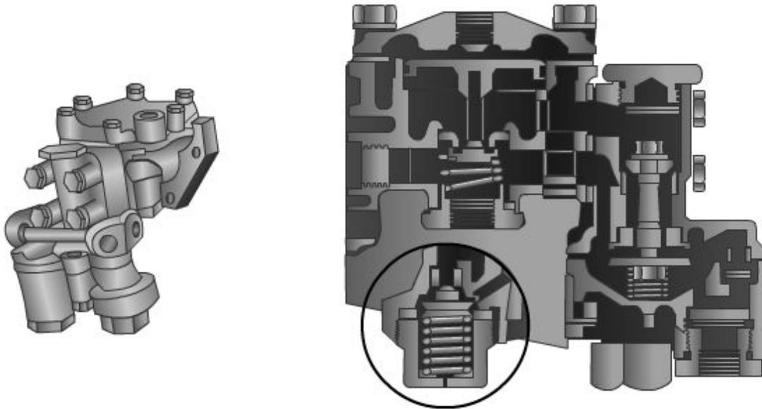
**Figure 13-38 — Relay emergency valve.**
