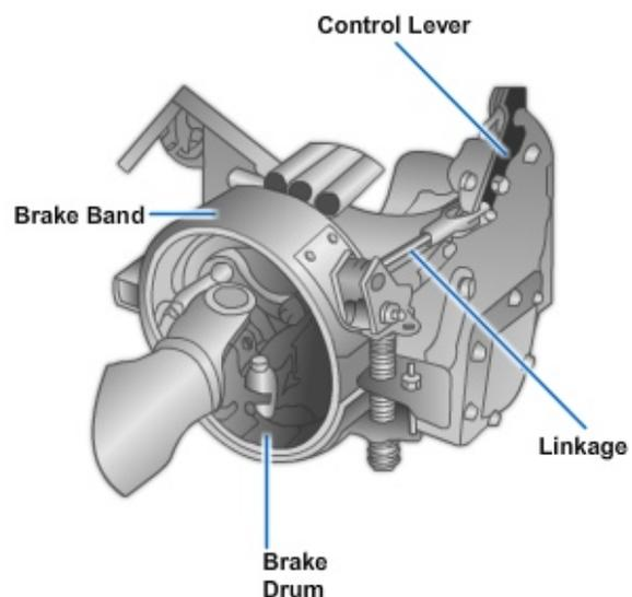
**Figure 13-20 — Transmission mounted emergency/parking brake.**
