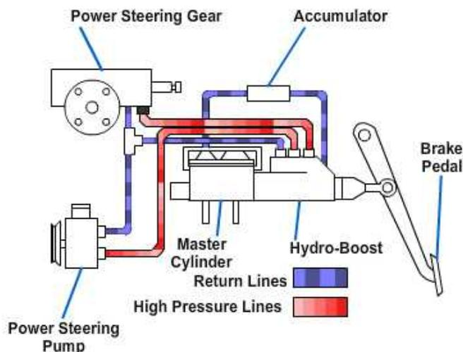
**Figure 13-17 — Hydraulic power booster system.**
