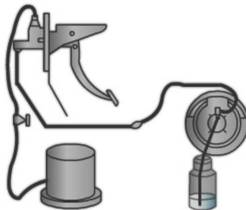
**Figure 13-23 — Pressure bleeding a brake system.**
