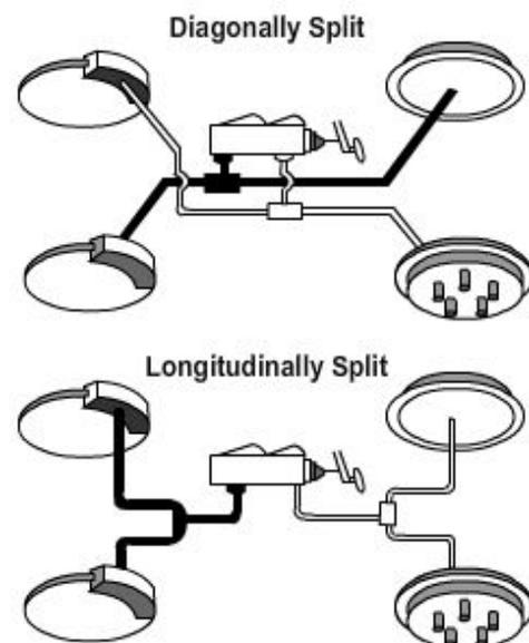
**Figure 13-4 — Dual master cylinder braking system.**
