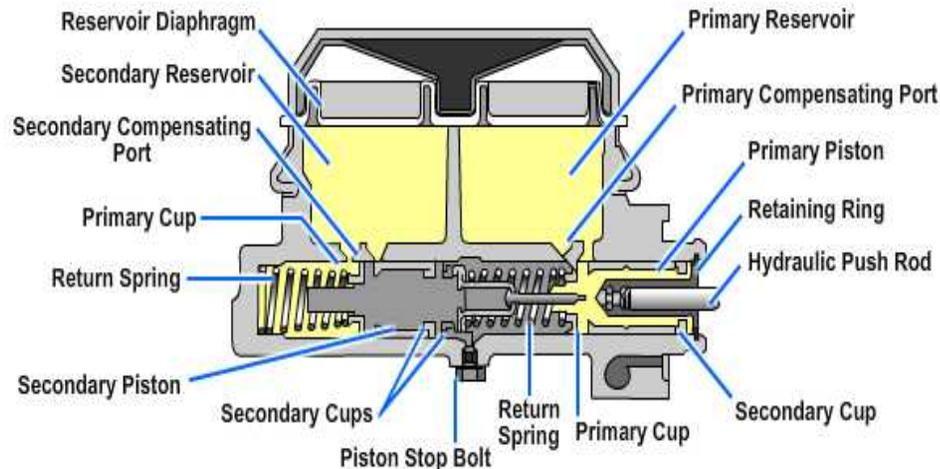
**Figure 13-3 — Cutaway view of a dual master cylinder.**
