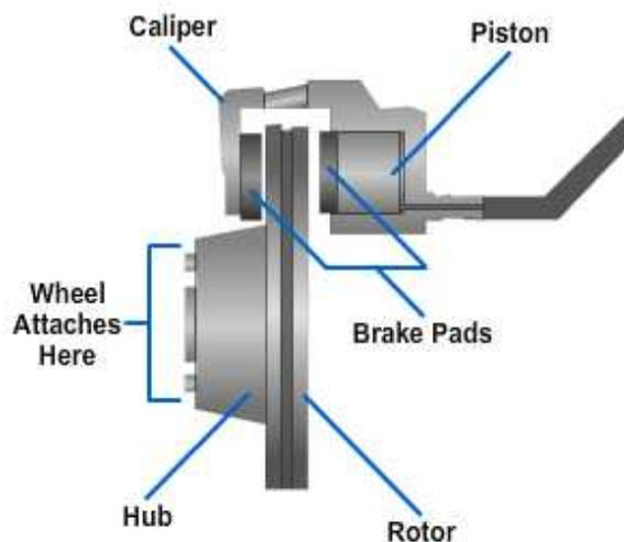
**Figure 13-12 — Floating caliper.**
