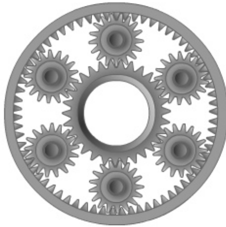
Figure 10-19 — Planetary gearset operation.
