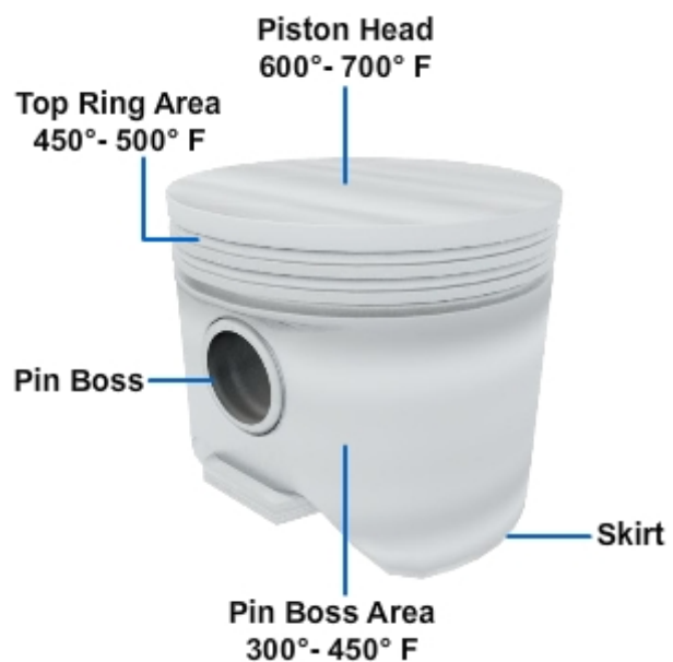
Figure 3-13 – Parts of a piston. 3-11
