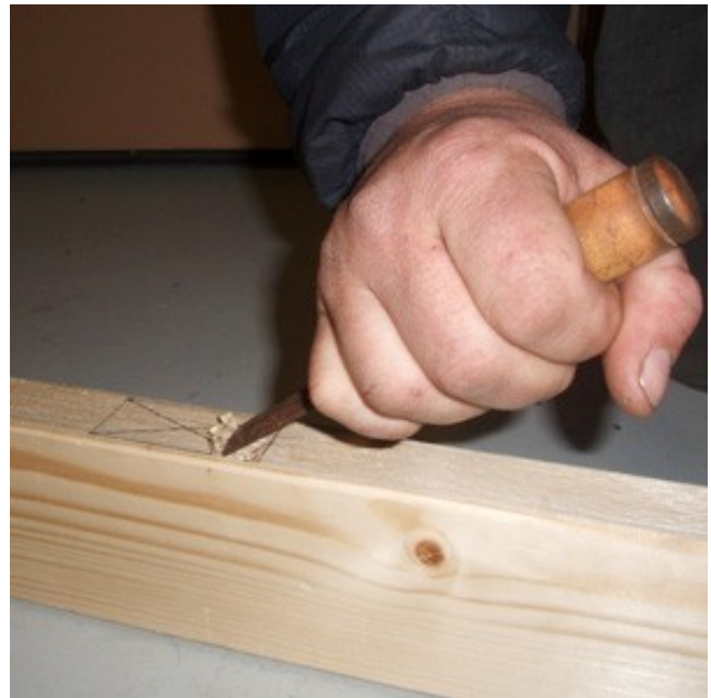
Figure 2-76 – Paring excess material with a chisel.
