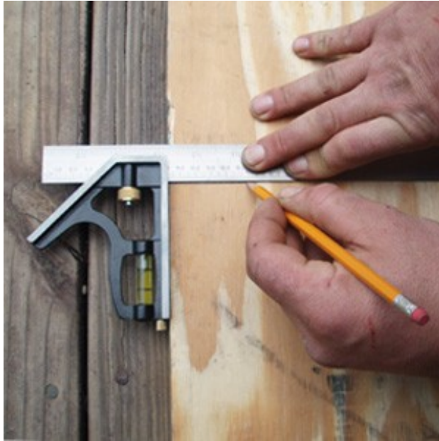
Figure 2-13 – Measure a 90° cut with a combination square.
