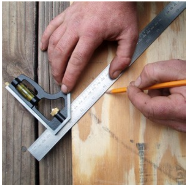
Figure 2-14 – Measure a 45° cut with a combination square.
