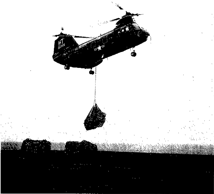
Figure 19.24. A CH-46 Sea Knight helicopter lowers cargo to the flight deck of an aircraft carrier during a VERTREP.
