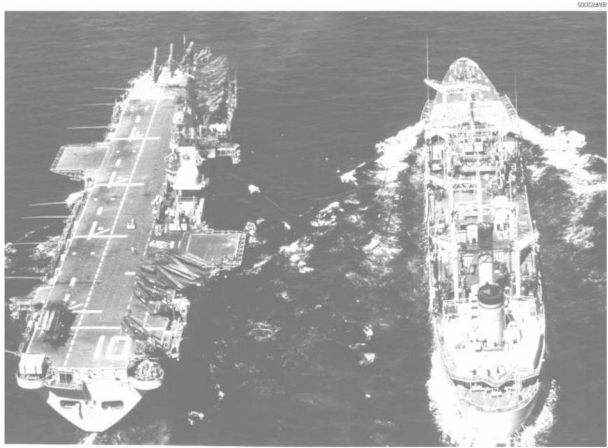
Figure 20-5.—Civilian-operated MSC oiler refueling an LPH.
