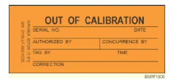
Figure 19-7.—Out-of-calibration label.
