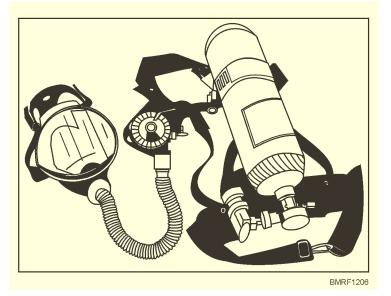
Figure 12-6.—Self-contained breathing apparatus (SCBA).
