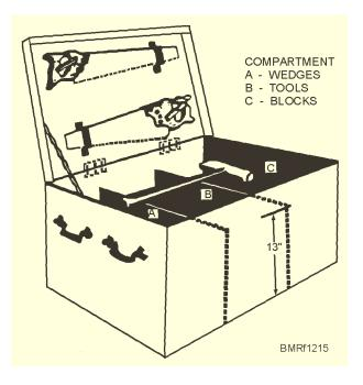
Figure 12-15.—Damage control shoring chest.
