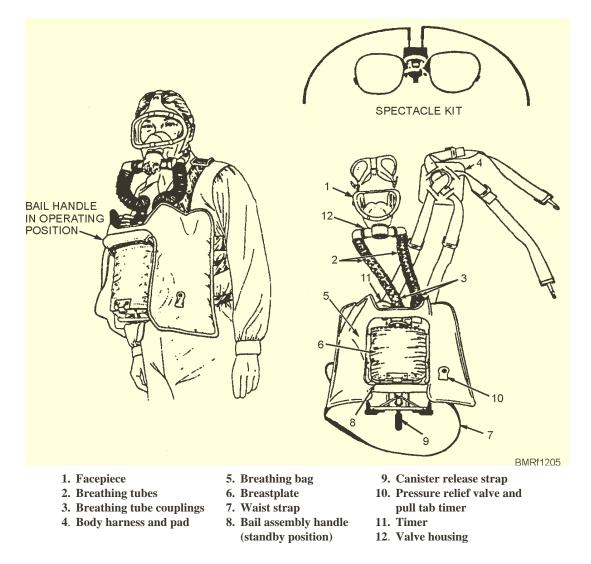
Figure 12-5.—Navy oxygen breathing apparatus (OBA).
