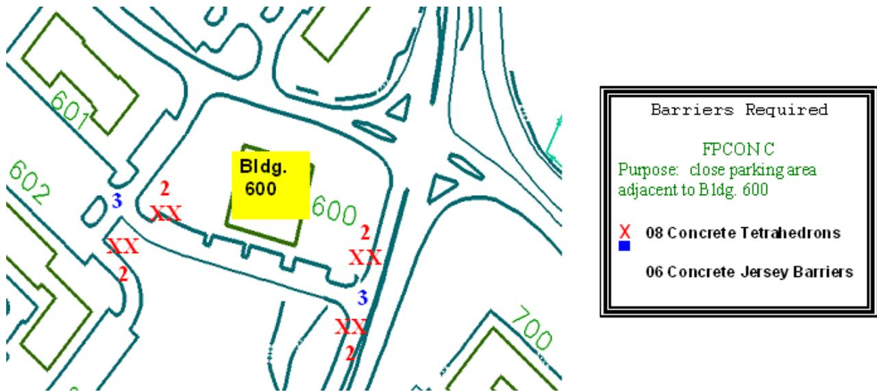
Figure B-2. Sample Drawing Showing Number and Type of Barriers
