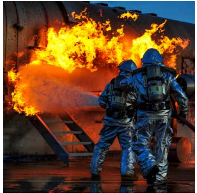
Sailors conduct firefighting training on an airfield using a Mobile Aircraft Firefighting Training Device, which can simulate 13 different aircraft fire situations. (U.S. Navy photo by Mass Communication Specialist 2nd Class Marcus L. Stanley/Released)
