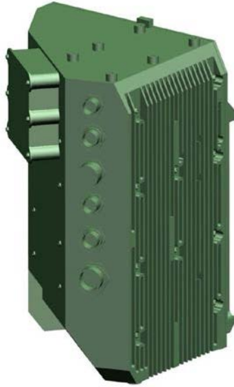
Figure 6. Power Electronics Assembly
