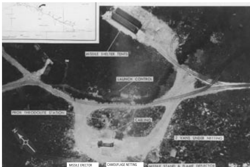
Anatomy of a crisis: At the top are the SS-5 missiles, housed in long tents. At the center is a launch control building, surrounded by service roads, missile erectors, and camouflage netting.
