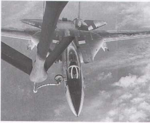
A Navy F-14 with a probe refuels from a drogue at the end of a KC-135's boom.
