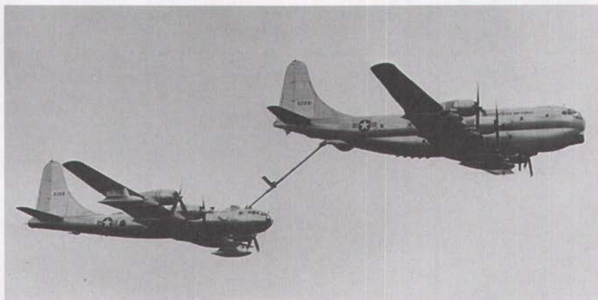
A KC-97 refueling a B-50. A comfortable aspect of this piston-engine pair was that both tanker and receiver used the same grade of fuel. The row of bumps on the underside of the KC-97's fuselage are lights that helped the receiver fly into proper position for refueling.
