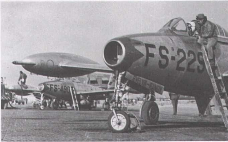
An F-84 with a wing tank fitted with a probe for refueling.
