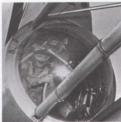
The earliest model of the Boeing boom was temporary, with exposed girders, cables, and pulleys. The boom operator in the KB-29P sat in what had been the tailgunner's space.
