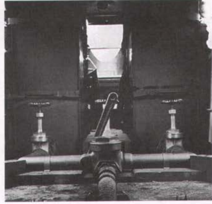
The cabins of the receiver (left) and the tanker. In the receiver, the fueling hose was placed in the funnel, which fed the cabin tanks under the duck boards at center. The tanker's refueling system has three gate valves, a levered quick closing valve, and a strainer in front of the hose.
