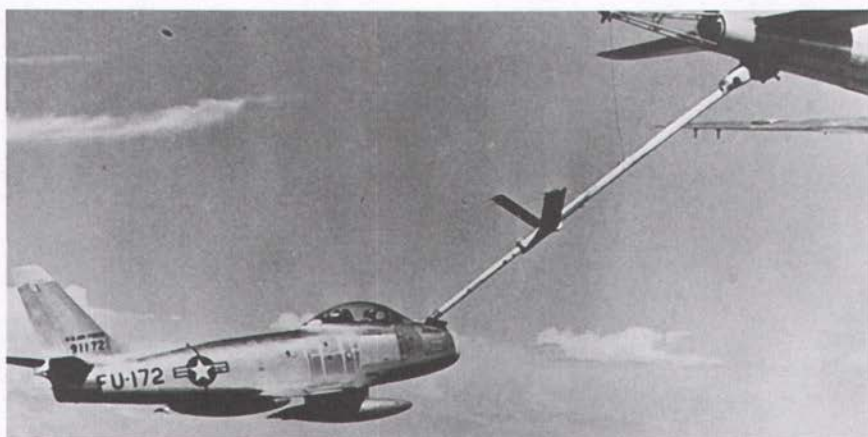
The F-101, one of the few airplanes designed with both systems, receives fuel from KC-97s through a drogue (top) and a boom (middle). Because of the F-86's internal structure, it was not fitted for inflight refueling. This F-86 (bottom) had to have its gun radar removed to create space for a refueling receptacle. No production F-86 models were refuelable.
