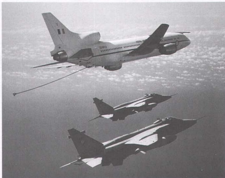
An RAF Lockheed L-1011 Tristar tanker trails a refueling drogue for Jaguar fighters. The probe over the nose allows the Tristar to be refueled in flight.
