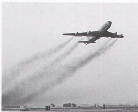
The KC-135’s original J57 engines were “smokers,” especially when water was injected to increase thrust (left). A B-52 maneuvers to connect with a KC-136 over Washington state in 1957.
