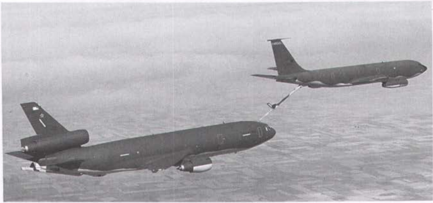
The McDonnell Douglas KC-10, here connected to a KC-135, is air refuelable, extending its range and versatility.
