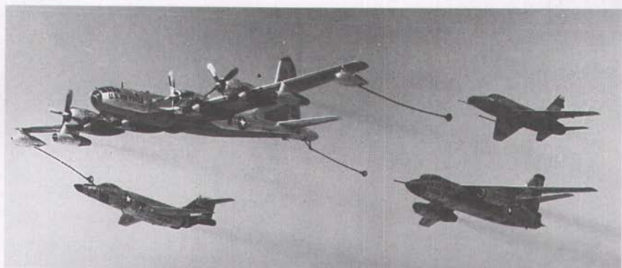
A TAC KB-50 trails three drogues for refueling. An RF-101 is connected (left), while a B-66 (center) and a F-100 (right) move up to connect.
