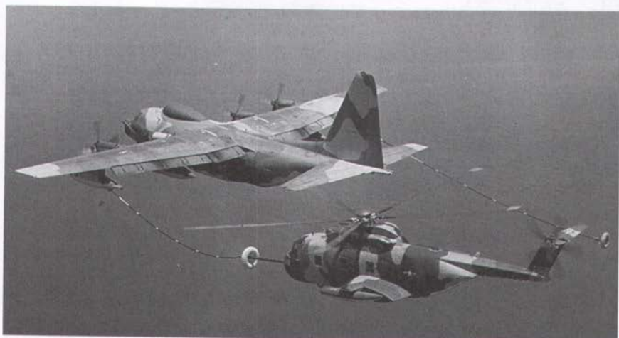
An HC-130, trailing two drogues, refuels an HH-3 over the Gulf of Tonkin.
