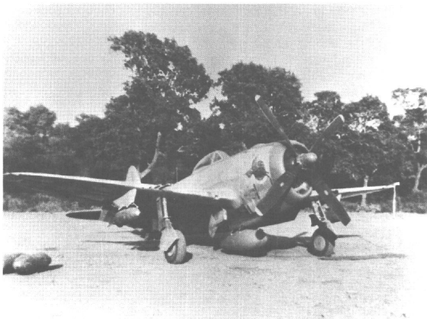
A Republic P-47D Thunderbolt shown with two 500-lb bombs and an external fuel tank, a typical offensive load carried in the 1944 campaign across France.
