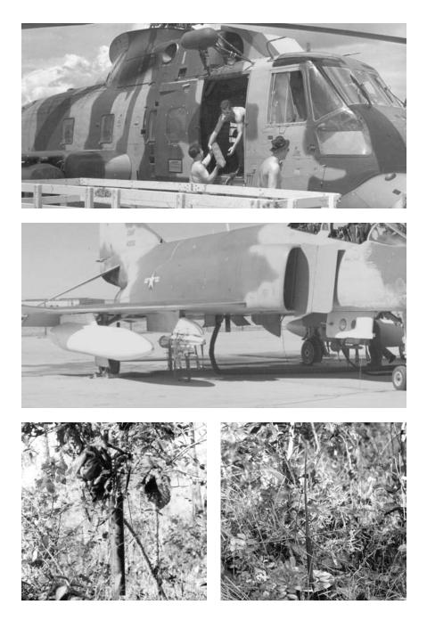
Acoustic sensors are loaded into a CH-3 (top), seismic sensors mounted on a pylon under an Air Force F-4 (center), an acoustic sensor hanging in brush (above left), and a seismic sensor embedded in the ground (above right).
