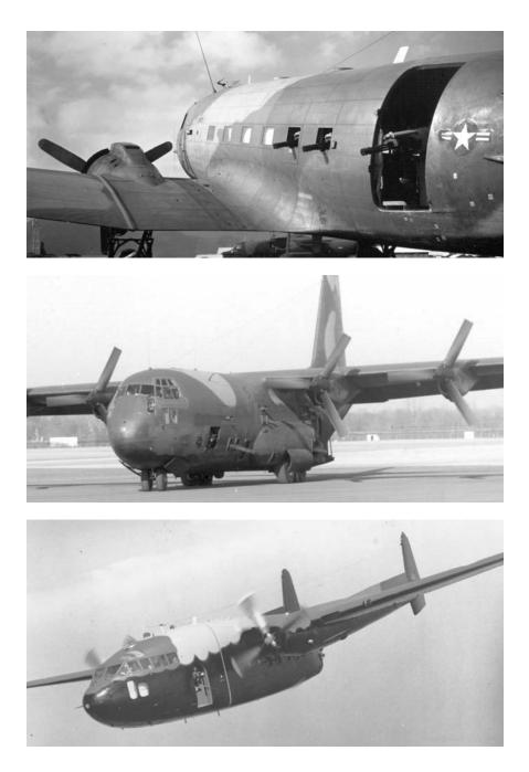
**Gunships**. Gunship I, an AC–47 (top ), carried three 7.62-mm miniguns; the Gunship II prototype, an AC–130A (center), had four 7.62-mm miniguns and four 20-mm guns; the AC–119G, Gunship III, (bottom), had four 7.62-mm miniguns.
