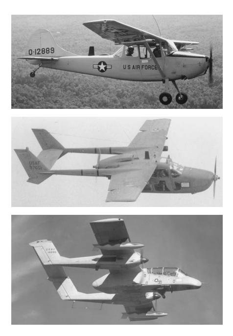
**Controller Aircraft.** Both the O–1 (top), which dated from World War II, and the twinengine O–2 (center) were modified commercial products. The twin-turboprop OV–10 (bottom) was designed for visual reconnaissance, was armored, and had hard points for armament. This one has a laser designator pod on the fuselage under the cockpit.
