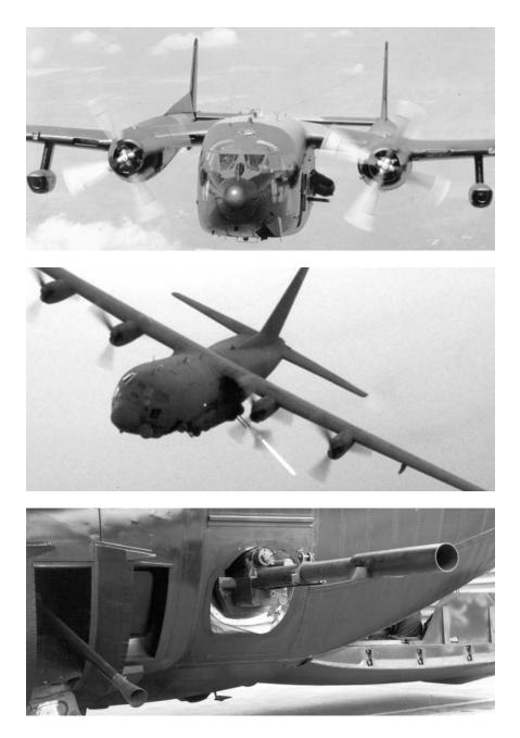
The second model of Gunship III, the AC–119K (top), had a jet engine under each wing and added two 20-mm guns. Later versions of the AC–130 carried two 40-mm Bofors guns(center) and a 40-mm Bofors and a 105-mm howitzer (bottom). Each improved gunship also had advances in numbers and types of on-board sensors.
