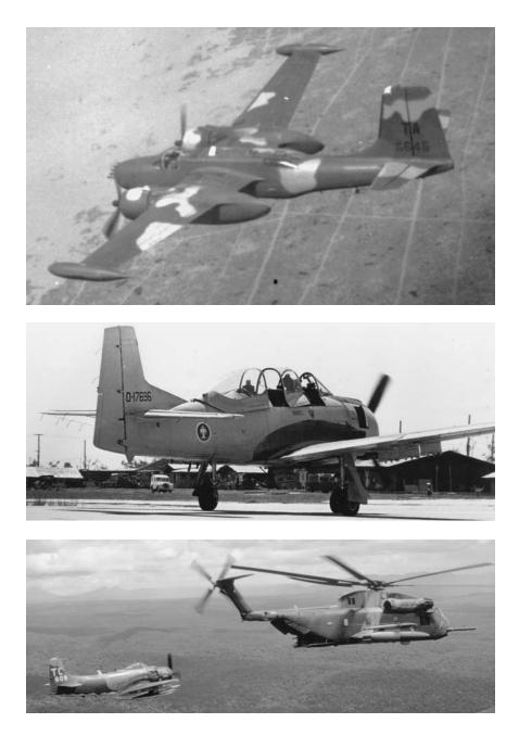
**Propeller Aircraft.** The A–26 (top) was one of the earliest aircraft attacking the Ho Chi Minh Trail in Laos. The T–28 (center), shown here with Laotian Air Force insignia, served in the air forces of several countries. The A–1 (bottom) filled many roles, here escorting an HH–53 rescue helicopter.
