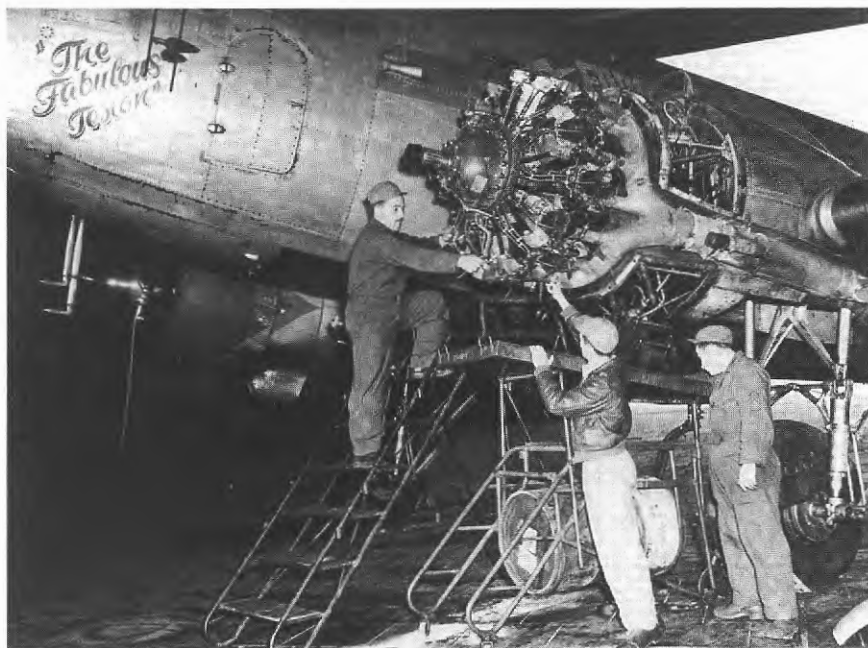
"Field maintenance." During unloading at Tempelhof, mechanics inspected engines and made minor adjustments. Here "The Fabulous Texan," a C-47, receives minor servicing. ( U.S. Air Force. )
