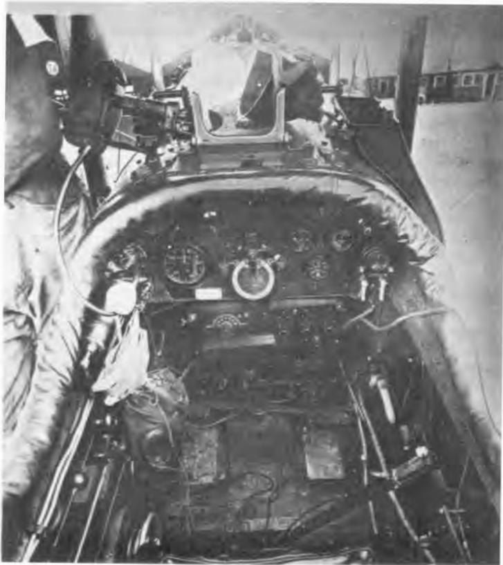
**Radio set installed in a DH-4.**
