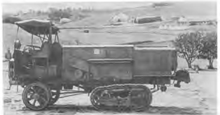
A balloon windlass mounted on a truck with a caterpillar adapter.
