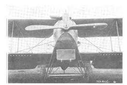
Loaded bomb rack on a Breguet.
