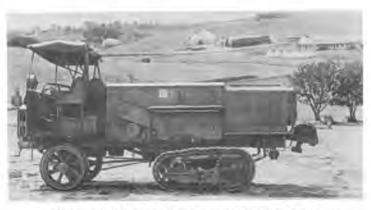
A balloon windlass mounted on a truck with a caterpillar adapter.
